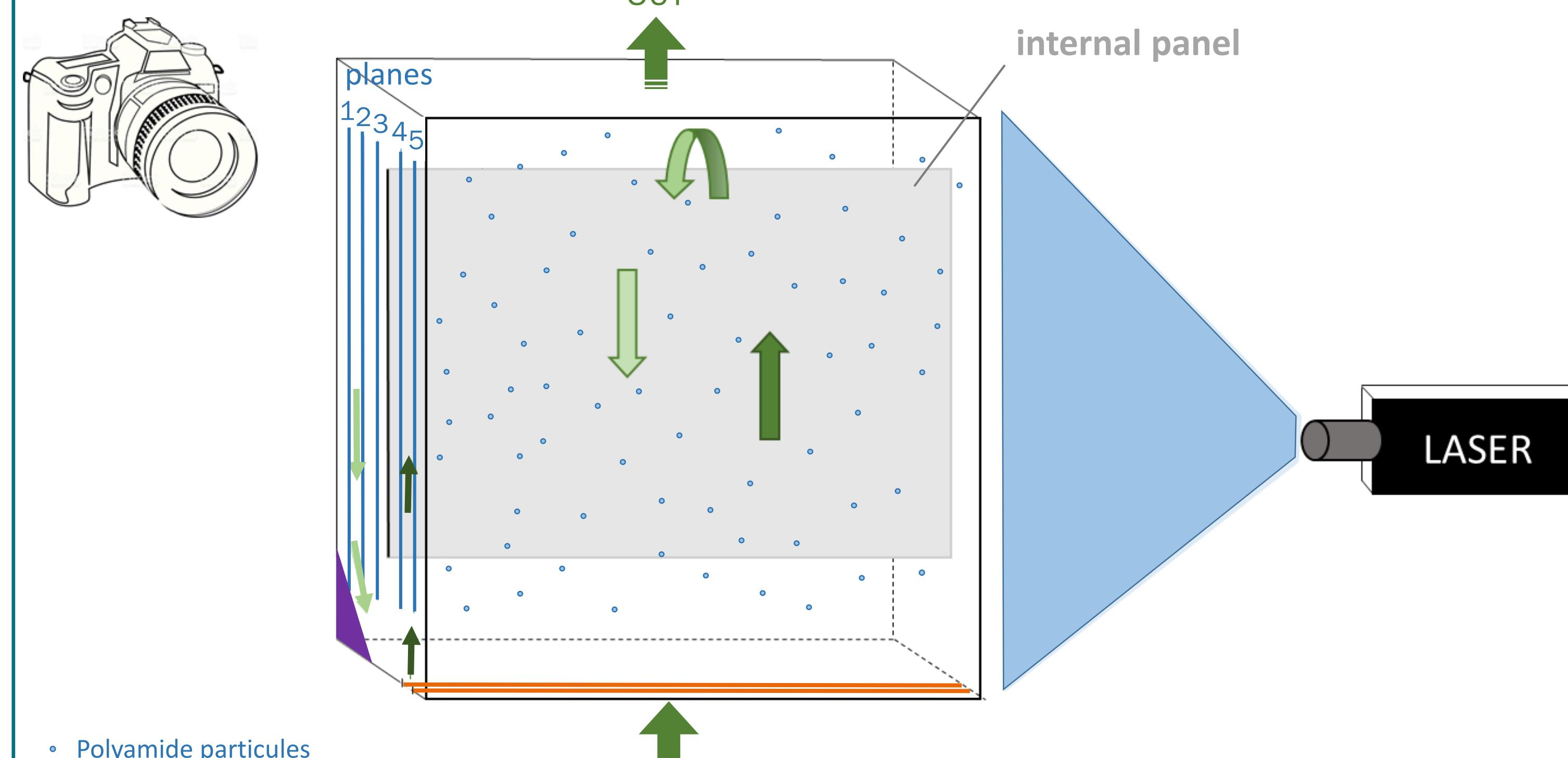
Bead recirculation improved by the internal panel, the off-center injection (1 mm) and the bottom prism
