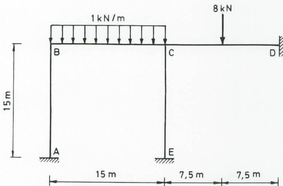
$$R : \quad M_A = -5,05 \text{ kNm}; \quad M_B(AB) = -M_B(BC) = -10,10 \text{ kNm}; \quad M_C(BC) = -20,87 \text{ kNm};$$
