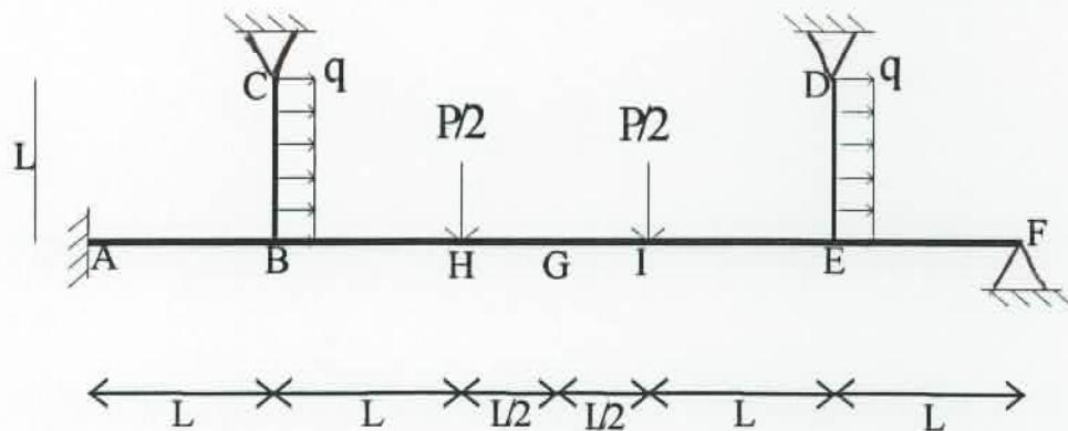
$$\begin{aligned}L &= 2 \text{ m} \\E &= 2,05 \cdot 10^8 \text{ kN/m}^2 \\P &= 100 \text{ kN} \\q &= 10 \text{ kN/m}\end{aligned}$$
