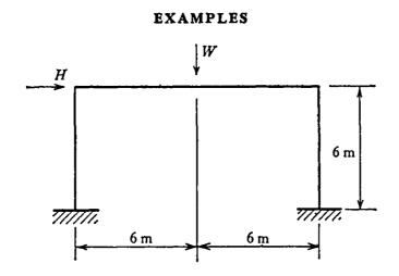
**2.41** In the figure the load factor,  $\lambda$ , and the plastic moment, M, are to be regarded as variables, as well as W, P, L and H. Plot, in the plane of the dimensionless variables  $(\lambda WL/M)$  and  $(\lambda PH/M)$ , the collapse locus for the family of loaded frames represented.
