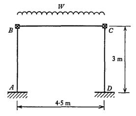
It may be assumed that a cross-section where the bending moment is less than  $66 \cdot 0$  kNm remains completely elastic, and that indefinitely large rotations can occur at constant moment at a plastic hinge.
