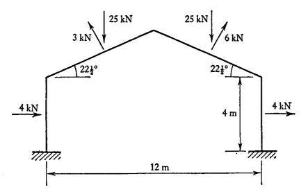
Estimate the required value of the full plastic moment so that the load factor against plastic collapse shall be 1.4. Instability effects and the reduction of plastic moments due to axial forces are to be neglected. (M.S.T. 11, 1953; adapted.) (Ans. 31.5 kNm.)
