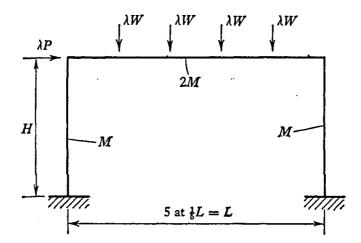
A frame conforming to the figure has H:L = 4:3. It is designed to a load factor of 2 under vertical loading only. What is the limiting value of P:W for this frame if under combined loading the load factor may be reduced to 3/2? (University of London B.Sc. (Engineering) Part III: Civil, King's College, 1965.) (Ans. 13:20.)
