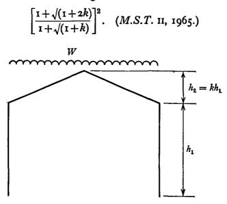
**2.52** The two-bay pitched-roof portal frame shown has members of uniform section of full plastic moment  $M_p$ . The rafters are connected to each other and
