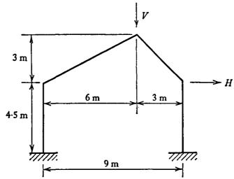
**2.50** A pitched portal with hinged feet is subjected to vertical loading of constant intensity  $\omega$  per unit horizontal distance, as indicated. The frame may be taken to have a plastic moment of resistance M throughout. Instability, and the effects on the plastic moment of axial and shear forces may be ignored.
