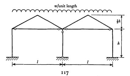
to the two external columns by full strength connexions. The external columns can sustain the full plastic moment at their feet, but the central column is a simple prop, pinned to the ground at one end and to the frame at the other. Light ties are connected across the frames at eaves level, and these are of sufficient section to prevent significant spread of the eaves when the frame is subjected to the factored collapse design load  $\lambda w$  per unit length, uniformly distributed.
