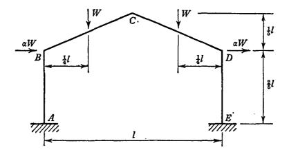
Investigate the value of W at which collapse will just occur for the load system shown. Present the solution in such a way that the mode of collapse and the value of W at collapse are indicated for any value of  $\alpha$ . Neglect the effect of the deformation of the structure on the equations of equilibrium. (M.S.T. 11, 1963.)
