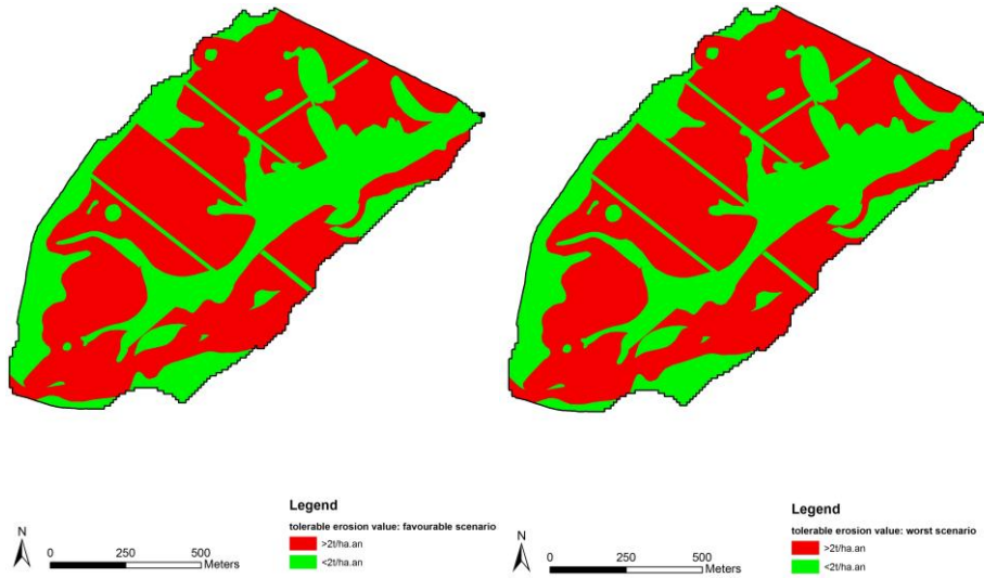
Figure IV- 18. Erosion values measured using the diachronic soil surveys method in relation to the JRC threshold for intervention.
