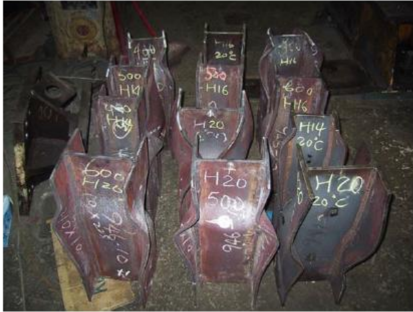
Figure 1: Failure of H-column specimens in the test programme carried out by Yang et al [11]
