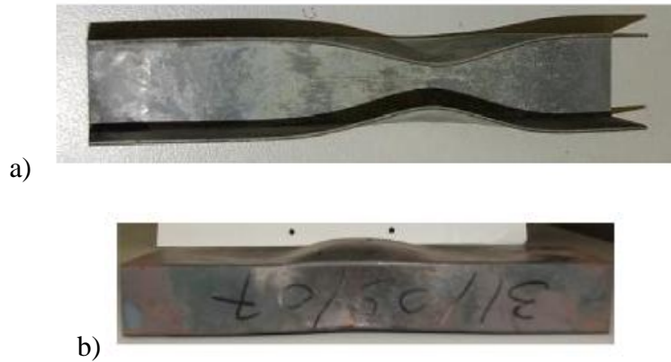
Figure 8: Typical local buckling failure a) of the flange b) of the web for cold formed steel specimens tested under fire exposure [40]
