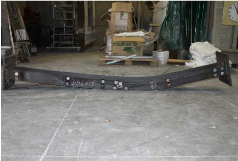
Figure 3: Global buckling of tested hot-rolled H-section after fire exposure [14]
