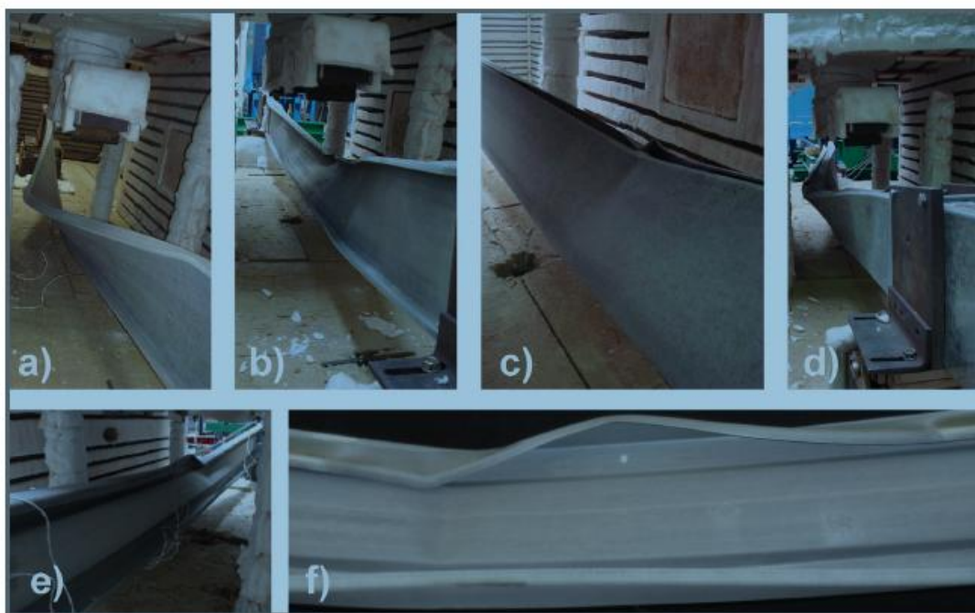
Figure 9: Failure of cold formed beams (a-f) involving local buckling after fire exposure [45]
