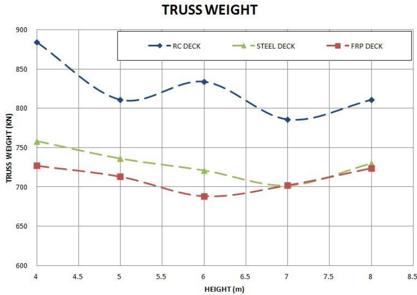
Figure 6. The single steel truss weight associated with each height at the center of the span.
