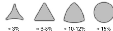
Variation of relative density of the foam with varying cross section profile: plateau, triangular, casting convex triangular and circular (used in most models); Duocel™ by ERG
