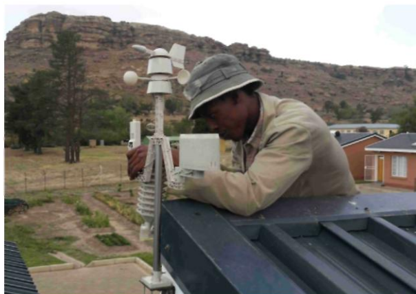
Fig. 5. Weather station installation at LDF health clinic by STG International staff (Makoanyane Khakhanyo).
