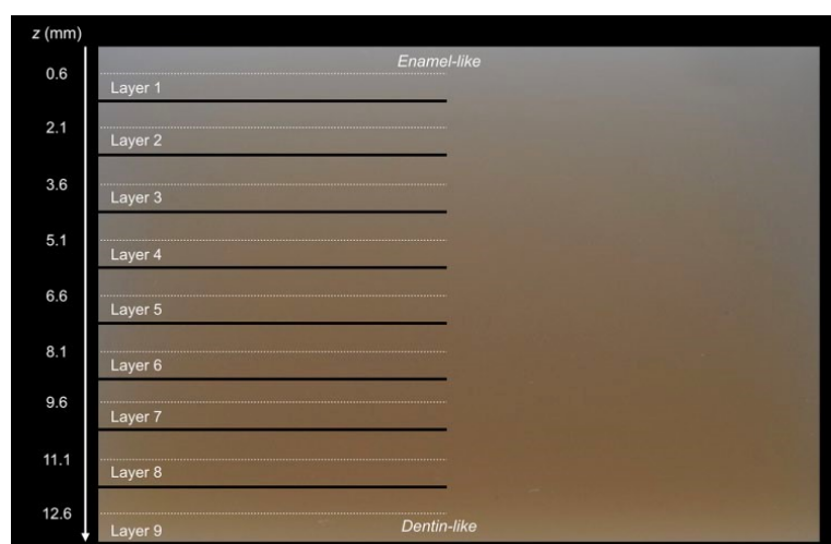
Figure 1. A functionally graded polymer-infiltrated ceramic network (FG-PICN) block with, on the left part, a schematic illustration of the cutting into 9 layers from the top (enamel zone) to the bottom (dentin zone). The black spaces between the layers represent the 0.3 mm of material lost during cutting (saw thickness). The thickness of each layer is (1.2 \pm 0.1) \text{ mm} ; measurements refer to the center of each layer (dashed line).
