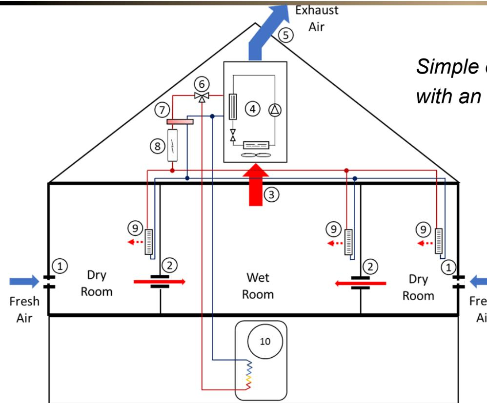
*Simple exhaust ventilation system combined with an exhaust air heat pump*
