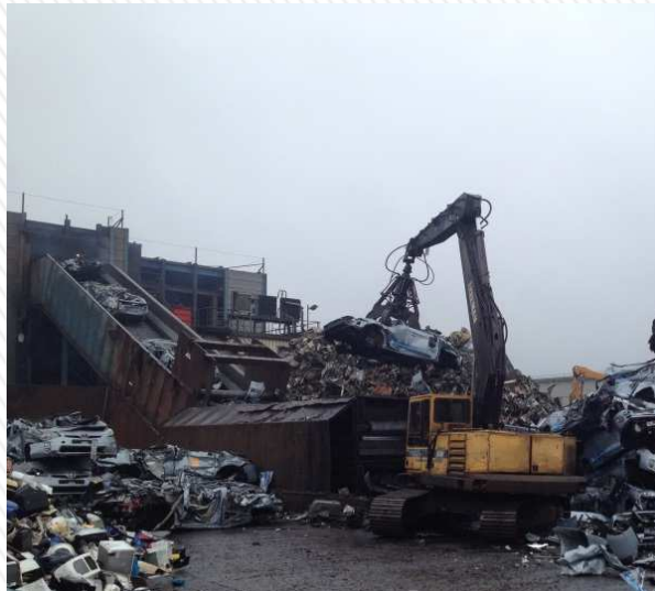
Loading the Shredder (5 ELV/min)
