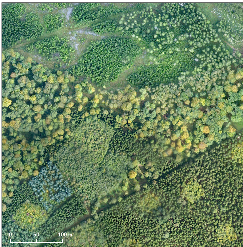
Figure 1.12: Example of Unmanned Aerial System (UAS) image at 25 cm resolution in East Belgium. The high spatial resolution allows to easily distinguish individual tree crowns and the spectral variations between trees.
