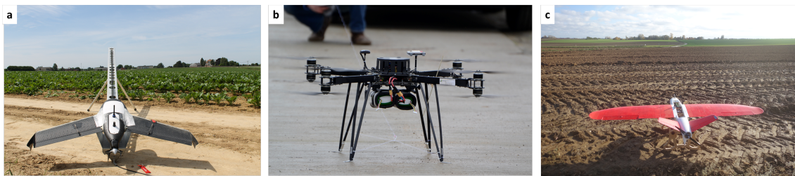
Figure 1.17: Three types of drones are used in Gembloux Agro-Bio Tech. (a) The Gatewing X100 used for the data acquisition in chapter 4 ;(b) An Multirotor, octocopter; (c) A fixed wing UAS.
