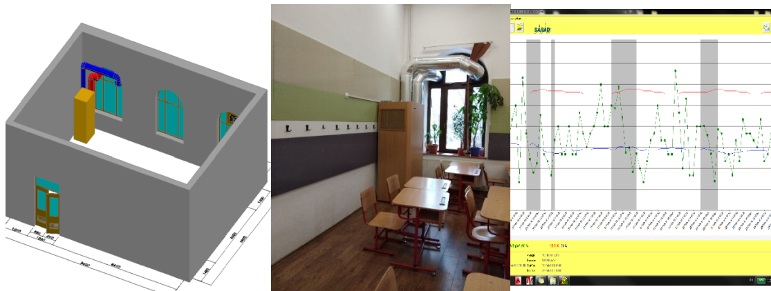
Figure 1 A 3D Model of the classroom B.Heat recovery ventilation unit photo C.Radon measurements
