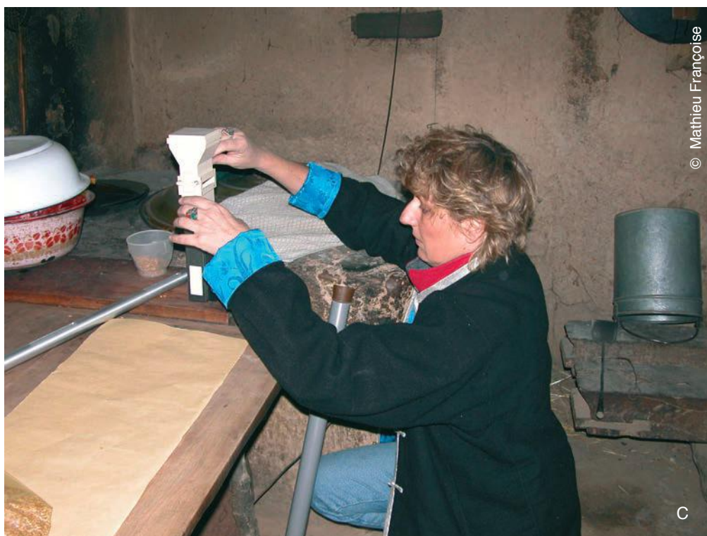
Plate 5.1. Surveys and samplings in the villages. A. Cereal grain are sampled in sacks or containers in the family store-room with a grain trier – B. This trier is conceived for sampling grain at different levels in bags or containers. It is important because fungal contamination may be different according the depth – C. Humidity of grain is also measured with a Samap device.
