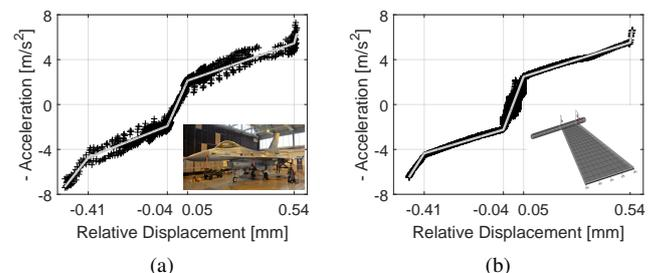
Figure 1: Qualitative stiffness curves computed by the ASM on (a) experimental results and (b) simulation results
