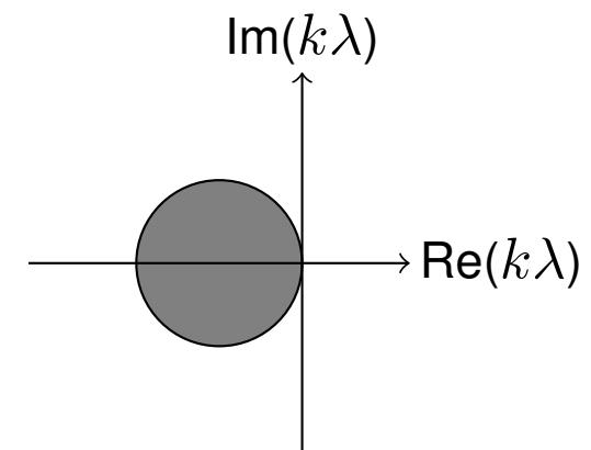
As a conclusion, the forward Euler method is conditionally stable. The time step  $k$  must be small enough for  $k\lambda$  to lie within the unit circle with center at  $(-1, 0)$  for the forward Euler method to furnish a numerical solution with the same asymptotic behavior as the exact solution.
