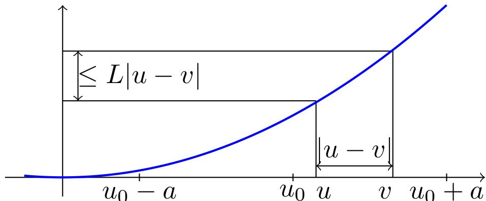
The function  $f(u) = u^2$  is Lipschitz continuous over any finite interval  $|u - u_0| \leq a$ , with  $L = 2(u_0 + a)$  if  $u_0 \geq 0$ .
