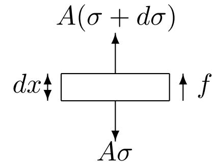
Here,  $u$  is the displacement,  $\epsilon$  the strain,  $\sigma$  the stress,  $A$  the cross section of the bar,  $E$  the Young's modulus, and  $f$  the external force per unit length.
