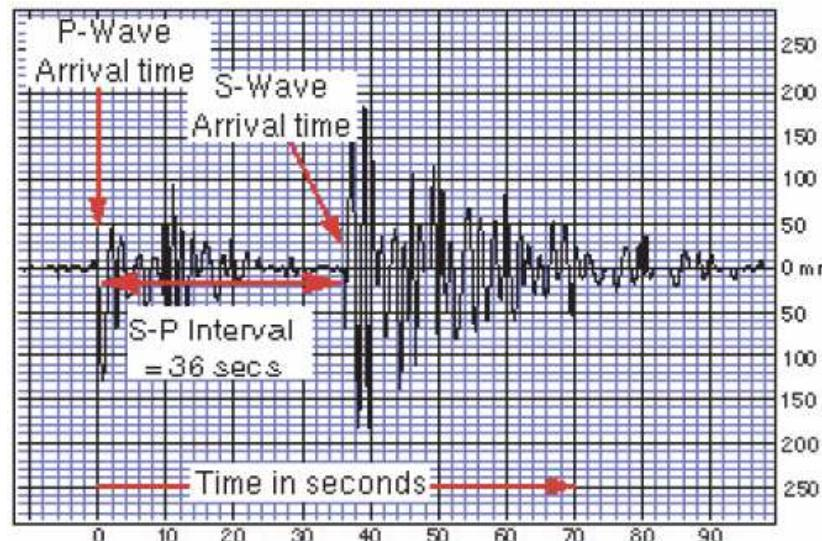
Given  $c_p$  and  $c_s$ , the length of the time interval between the arrival of the P and S waves after an earthquake allows the distance between the seismic recording station and the epicenter of the earthquake to be estimated. Repeating such an analysis for multiple seismic recording stations allows the location of the epicenter of the earthquake to be estimated.
