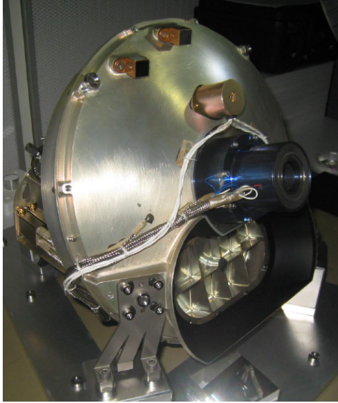
Figure 1.3: Picture of the calibration assembly of the UVN instrument integrated in the CSL clean room.
