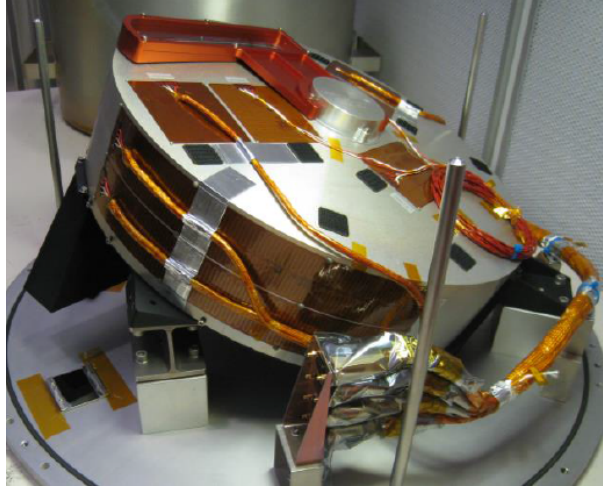
Figure 1.1: Picture of the calibration assembly of the OLCI instrument integrated in the CSL clean room [12].
