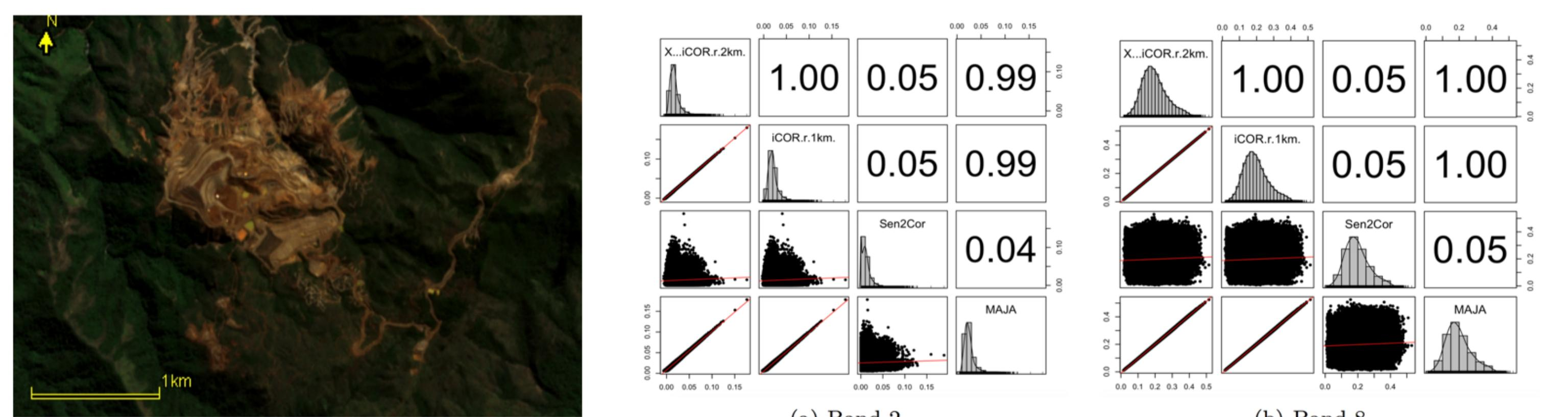
**2- Fusion of various sources of data with Sentinel 2 to accomplish mapping of iron-oxide and its bearing dust.** Using hyperspectral acquisitions and chemical composition of field samples, regression models can be developed to map mining sites and outcrops. The example below shows an outcrop in Thiebaghi, New Caledonia (False color Sentinel 2 image of 11<sup>th</sup> of February, 2018) and its iron-oxide content.
