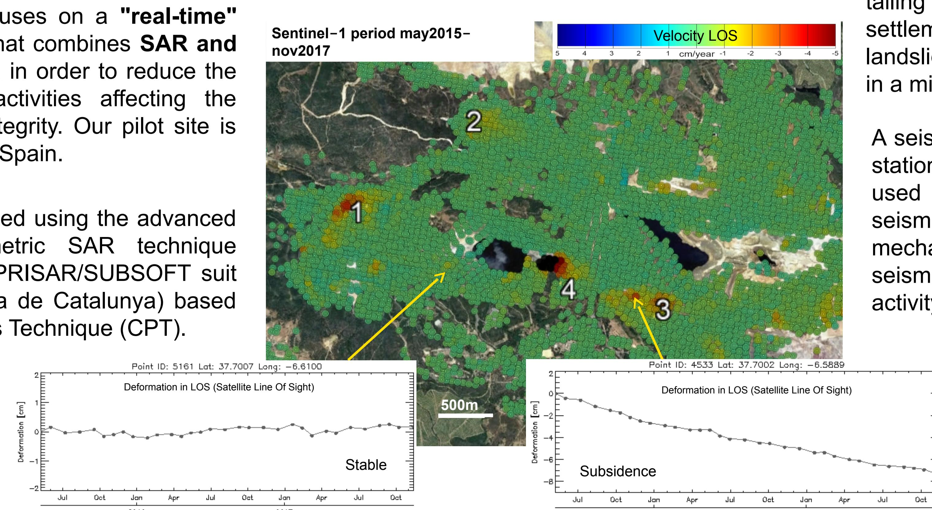
We have identified four deformation zones (left). Zone 1, 2 and 3 are tailing zones showing subsidence patterns (warm colors) due to settlement. Zone 4 is the eastern wall of an abandoned pit affected by landslides. Thus, Sentinel-1 is a good tool for monitoring soil integrity in a mine context.
