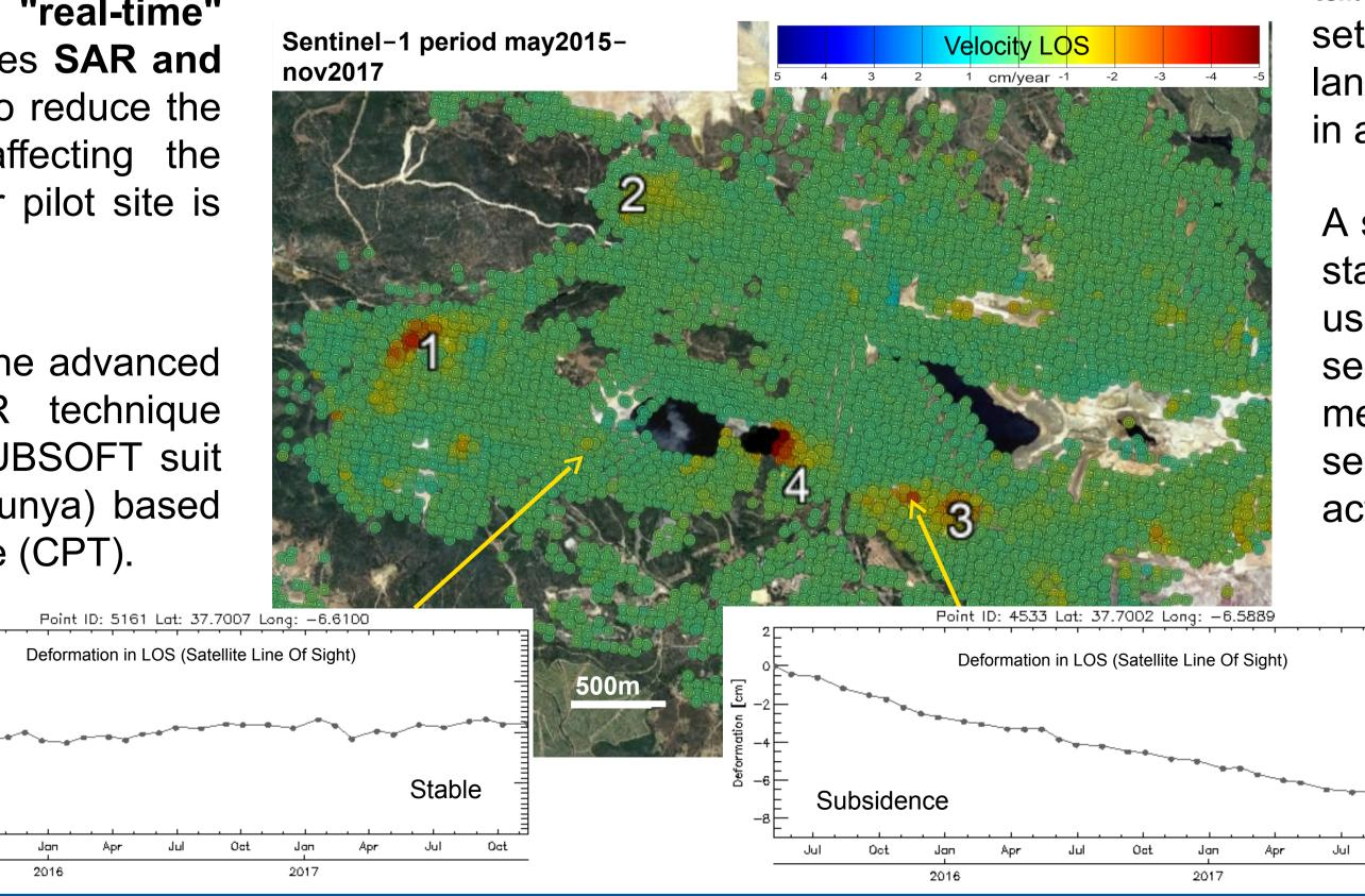
We have identified four deformation zones (left). Zone 1, 2 and 3 are tailing zones showing subsidence patterns (warm colors) due to settlement. Zone 4 is the eastern wall of an abandoned pit affected by landslides. Thus, Sentinel-1 is a good tool for monitoring soil integrity in a mine context.
