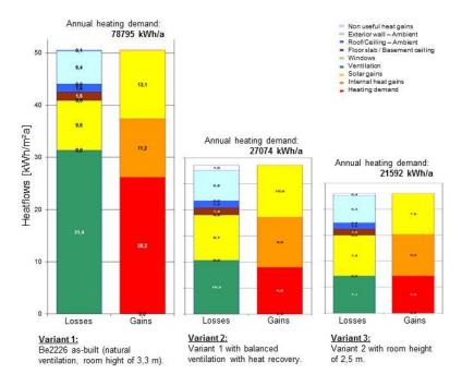
Fig. 2: Relation between ceiling high and energy balance heating of be2226 according to the Passive House Planning Package (PHPP) [4] (Author)
