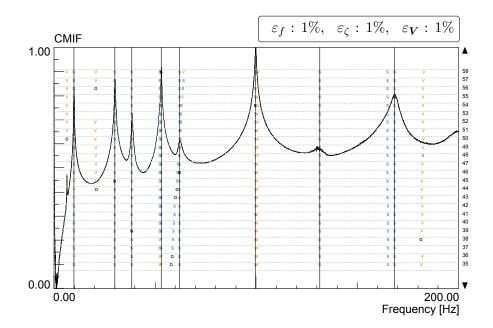
Figure 4.2: Stabilization diagram of the beam subsystem. The selected poles are appear as bold black  ${\bf s}.$
