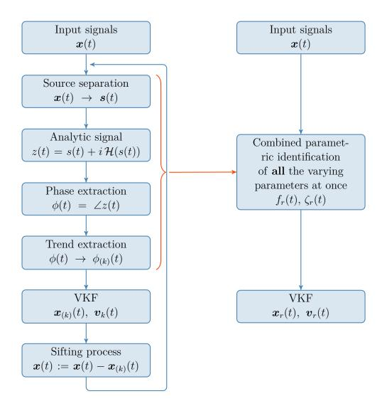
Figure 2.1: Graphical representation of the methodology for the identification of timevarying systems.
