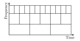
Figure 1.4: Illustration of the wavelet transform.
