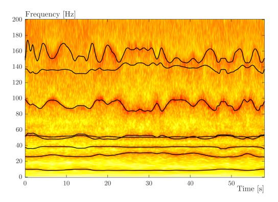
Figure 4.16: Time-varying frequencies identified with a basis of functions based on the position of the mass.
