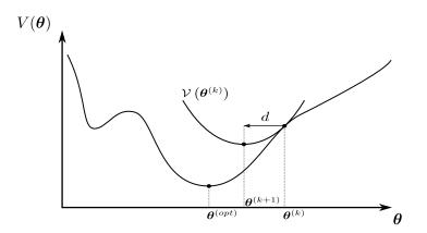
Figure 2.2: Illustration of the Newton approach. At iteration k, a quadratic model of the function is built based on the gradient and Hessian information. It is then minimized to give the next set of parameters.
