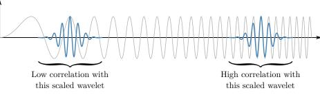
Figure 1.3: Illustration of the wavelet transform.
