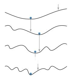
Figure 3.8: Illustration of the path to the solution by graduated optimization.
