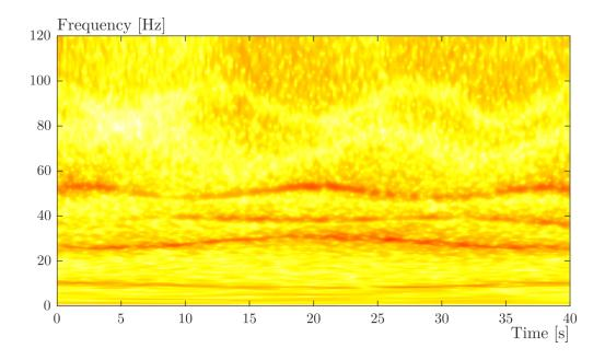
Figure 1.28: Residual after the first extraction of the fifth time-varying mode on the second sensor measurement.
