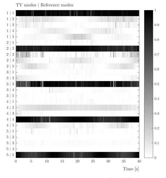
Figure 1.34: Time-varying modal assurance criterion (TV-MAC). The y-axis label indicates the couples of modes which are compared and the time dependency appears along the x-axis.
