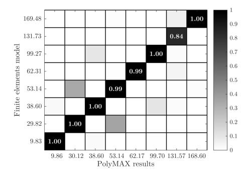
Figure 4.4: MAC matrix between the identified LTI structure and its basic finite element model.
