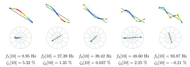
Figure 3.6: Snapshots of the five physical modes at t = 10 s with their shape, Argand representation and frequency and damping ratio information.
