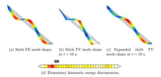
Figure 4.13: The expansion process of the experimental time-varying modes is illustrated to match the finite element mesh.
