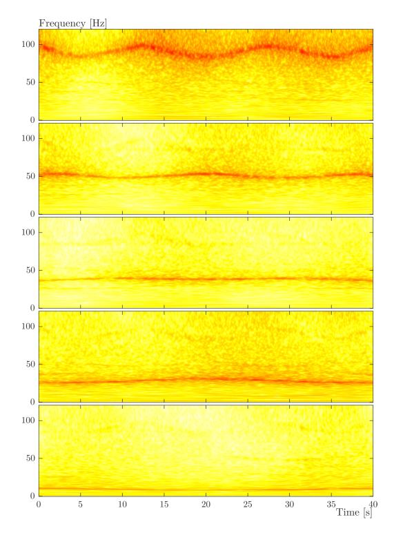
Figure 3.11: The modal contribution of each mode is a direct product of the modal domain state-space identification. Time-frequency representations of the five modal contributions of the second channel are shown.
