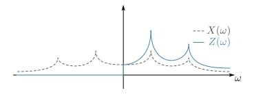
Figure 1.8: Specra of a signal and its correspondent analytic signal.
