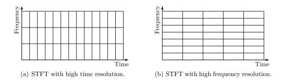
Figure 1.1: Illustration of the trade-off between time and frequency resolution in the STFT.
