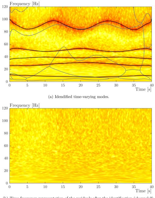
(b) Time-frequency representation of the residuals after the identification (channel 2).
