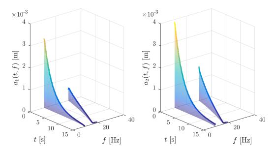
Figure 1.19: Hilbert spectra of each components after the decomposition by the HVD method preceeded by the source decomposition.
