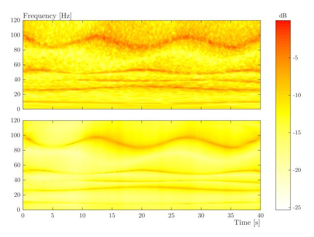
Figure 2.14: Comparison of the time-varying PSDs between nonparametric and modelbased approaches. Top: scalogram with the wavelets spectrum, bottom: computed with (2.87).
