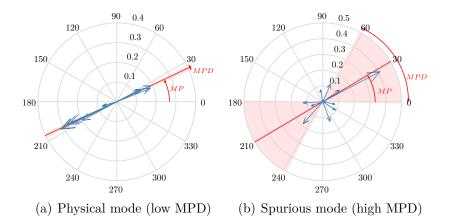
Figure 3.4: Illustrative example of the mode phase dispersion in the complex plane. (a) is a physical mode and (b) is classified as a spurious.
