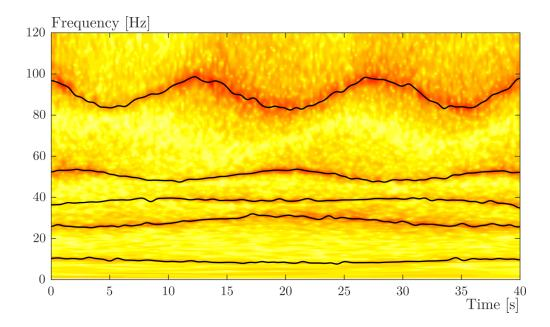
Figure 1.32: Final set of instantaneous frequencies. All the modes are identified in the frequency band.
