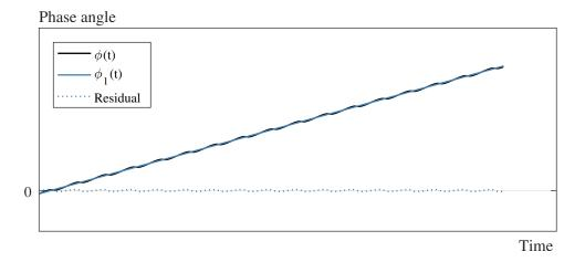
Figure 1.20: The phase angle of a multicomponent analytic signal dominated by the phase of the dominant component.
