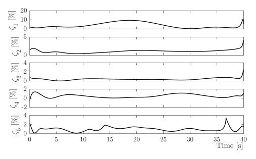
Figure 2.8: Time-varying evolution of the frozen damping ratio's of the structure corresponding to the identified frozen poles.
