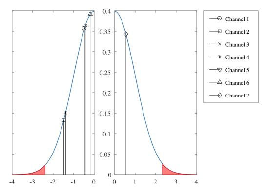
Figure 2.9: Sign test validation for the residual sequences in each measurement channel. The rejection criteria is fixed at 1% chance to have less or higher runs in each distribution tail.
