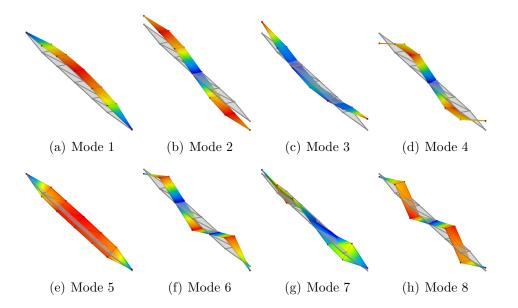
Figure 4.3: Complete set of mode shapes up to 200 Hz in the linear time invariant case.
