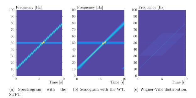
Figure 1.6: Illustration of different time-frequency representations for a multicomponent signal.
