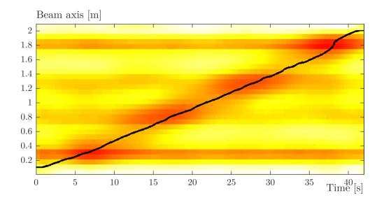
Figure 4.14: Estimation of the position of the mass by the deviation in elementary kinematic energies.
