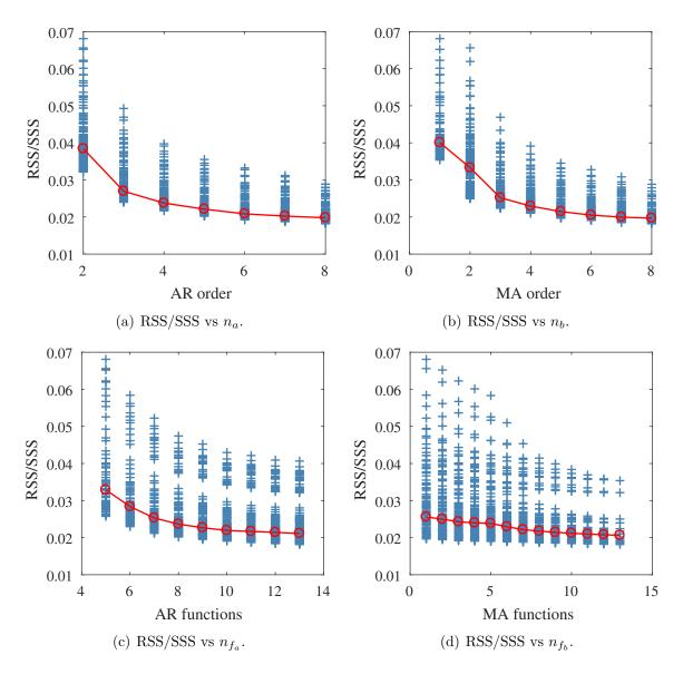
Figure 3.2: RSS/SSS values with respect to each of the model structure parameter of the ARMAV model.
