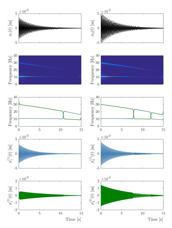
Figure 1.16: Time responses and extracted instantaneous frequencies and components. First row: time response of each DoF. Second row: Wavelet plots of each response. Third row: identified instantaneous frequencies for each DoF by the HVD method. Fourth and fifth rows : monocomponents corresponding to the each identified instantaneous frequencies.
