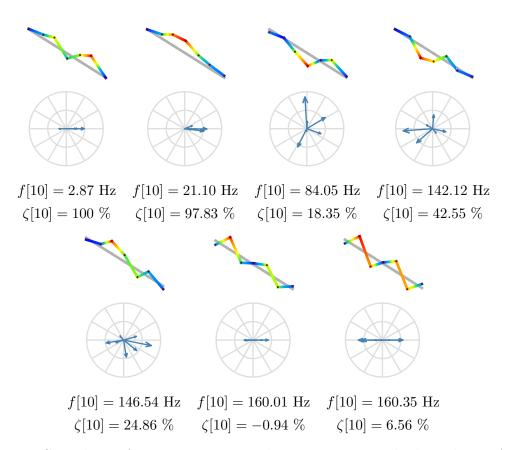
Figure 3.7: Snapshots of seven spurious modes at t = 10 s with their shape, Argand representation and frequency and damping ratio information.
