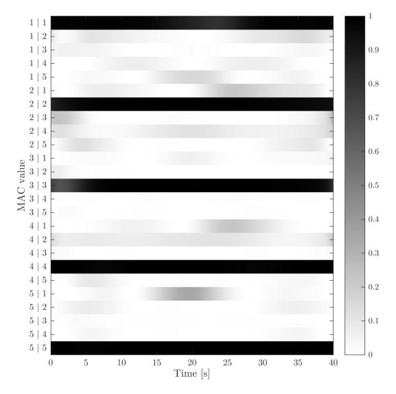
Figure 3.13: Comparison in mode shapes between the two kinds of models with the full TV MAC matrix.
