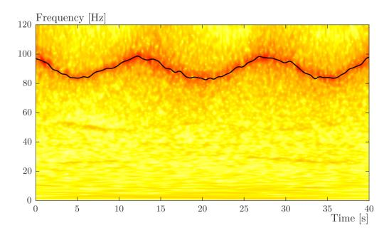
Figure 1.27: Wavelet spectra of the first selected source computed by the SOBI method. The dark line corresponds to the computed instantaneous frequency of its dominant component.
