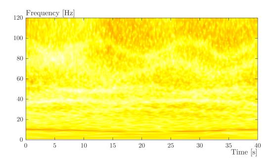
Figure 1.30: Residual after the extraction of the extraction of four identified modes.
