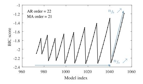
Figure 2.5: Zoom on the BIC criterion for the model structure with AR and MA orders fixed at 22 and 21, respectively. The variations of the BIC values are due to the increase in both  $n_{f_a}$  and  $n_{f_b}$ .
