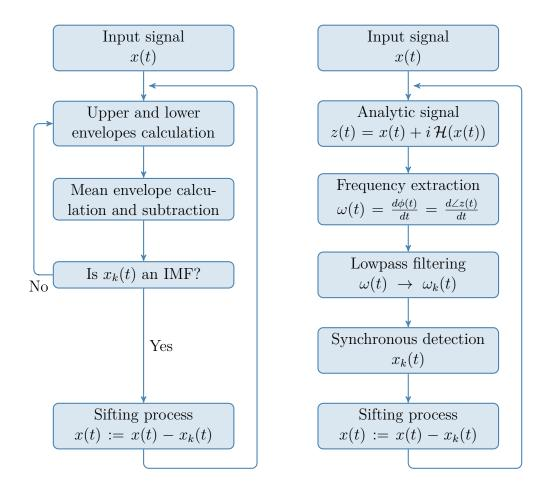
Figure 1.13: Comparative block diagram representations of the EMD (left) and HVD (right) methods.
