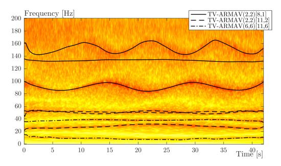
Figure 4.9: Combination of three model structures for the full identification.
