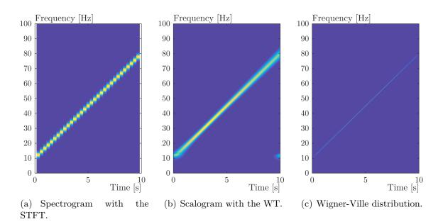
Figure 1.5: Illustration of different time-frequency representations.
