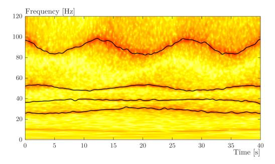
Figure 1.29: Instantaneous frequencies identified by the method after four iterations. The lowest frequency mode has a comparable amplitude with the remaining noise at higher frequencies.
