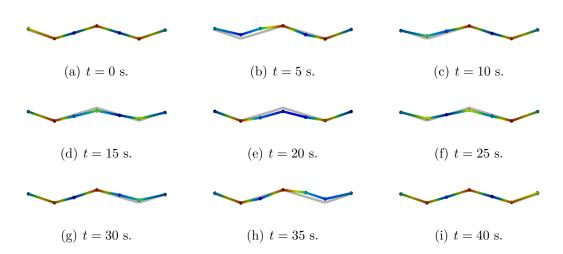
Figure 1.36: Fifth time-varying mode shape at equally spaced time spots. The starting position of the mass is on the left hand side of the beam and travels to the right. The background grey shape represents the mode shape of the LTI structure.
