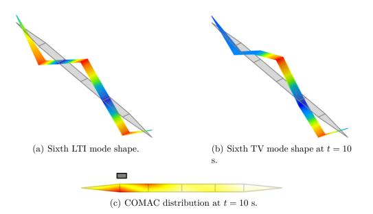
Figure 4.11: Comparison between the reference experimental set of modes and the time-varying identified ones with the *COMAC* criterion. The gray rectangle represents the actual (recorded) position of the mass.
