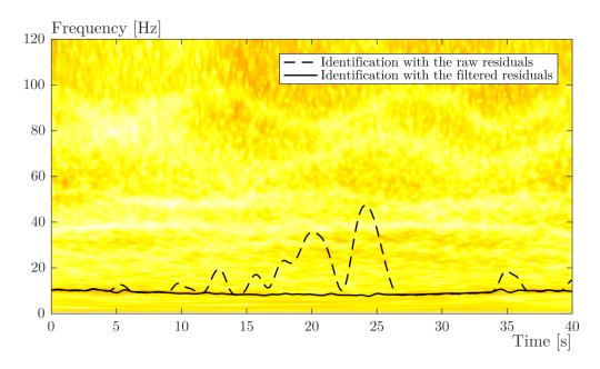
Figure 1.31: Identification of the lowest time-varying frequency by processing raw or filtered residual. The the wavelet decomposition of the raw residual is used as background support.
