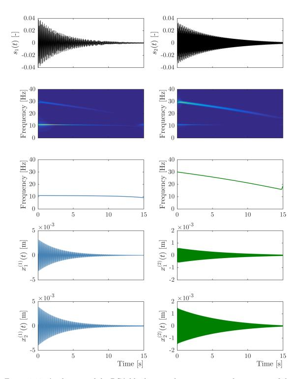
Figure 1.18: Application of the PCA blind source decomposition and extraction of the instantaneous frequency of their dominant component. First row: time evolution of each source. Second row: Wavelet plots of each source. Third row: identified instantaneous frequency of the dominant component. Fourth and fifth rows : monocomponents corresponding to the identified instantaneous frequencies in each channel.
