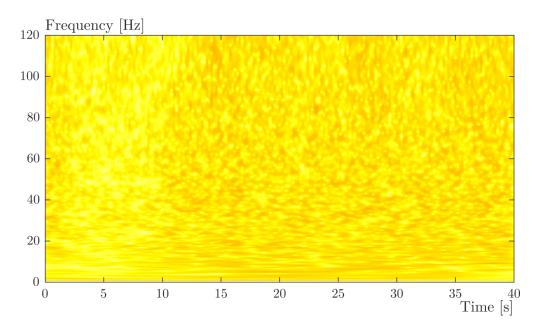
Figure 2.10: Time-frequency representation of the residual sequence of the second channel. Each active mode in the frequency band of interest is properly modeled and extracted from the measurement data.
