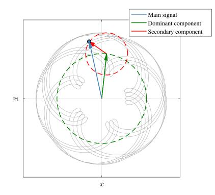
Figure 1.12: Trajectory in the phase plane (real versus imaginary part) of the analytic signal with two components. The gray track represents the trajectory of the combined signal and the green and red vectors represent the phasors of the two monocomponent signals.
