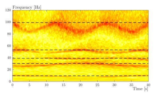
Figure 1.26: Wavelet spectra of the response of the second sensor. The dashed lines represent the natural frequencies without considering the additional mass (Table 1.1).
