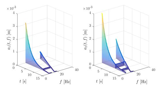
Figure 1.17: Hilbert spectra of each components after the decomposition by the HVD method.
