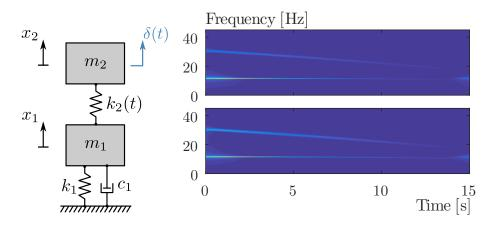
Figure 1.15: Simple 2 DOFs system submitted to an impulse.
