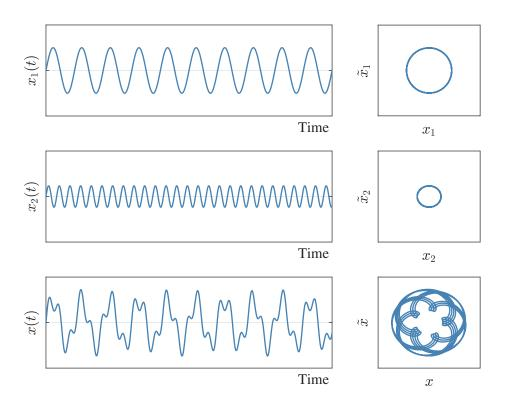
Figure 1.9: Signal composed of two different monocomponents.
