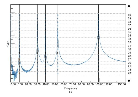
Figure 1.25: Stabilization diagram obtained using the PolyMAX identification on the reference beam.
