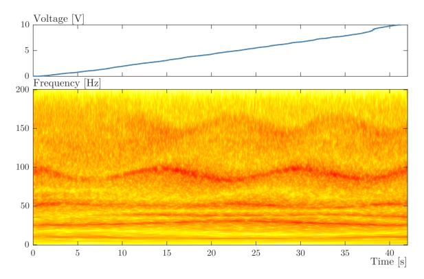
Figure 4.5: Time-frequency representation of the time-varying response in the third channel. The relative position of the center of the mass is plotted on the top.
