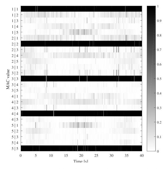
Figure 2.12: Time-varying modal correlation between the time-varying modes obtained with both methods.
