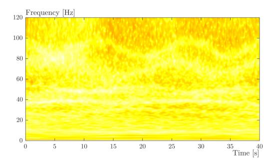
Figure 1.33: Residual signal in the second channel after the extraction of each monocomponent related to the identified instantaneous frequencies.
