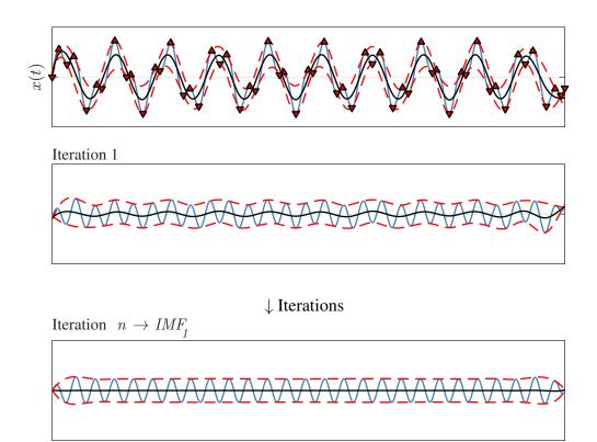
Figure 1.11: Illustration of the slow oscillation removal from the initial signal until only the fast oscillation component remains.
