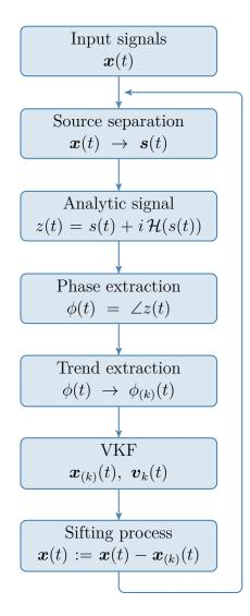
Figure 1.22: Flowchart of the modified HVD method.
