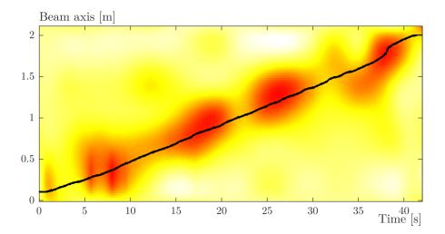
Figure 4.12: Estimated position of the mass by the COMAC criterion. The black line represents the measured position of the mass.
