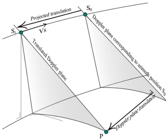
Figure 6. Geometrical iterative process for inverse projection
