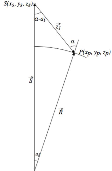
Figure 3. SAR viewing geometry
