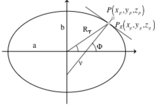
Figure 2. Geodetic height
