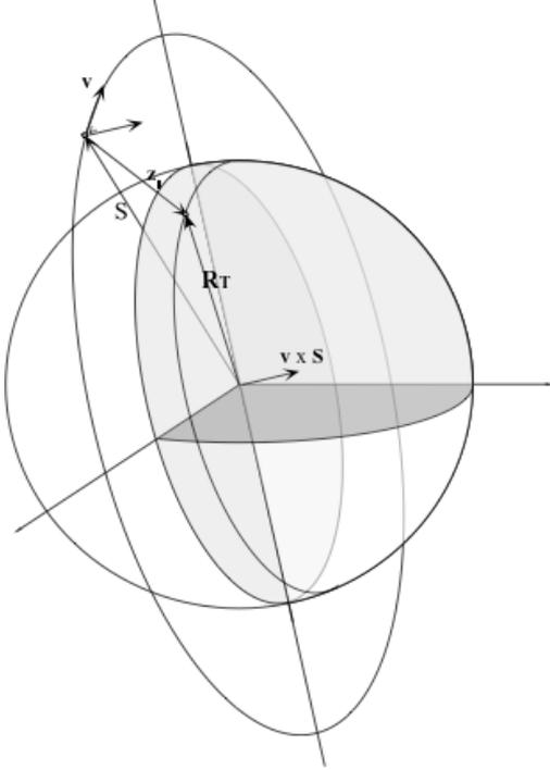
Figure 4. Right-side looking SAR sensor
