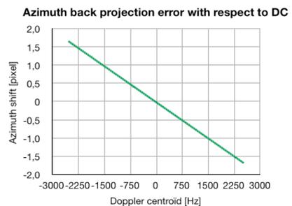
Figure 7. Azimuth back projection error with respect to DC using a single iteration.
