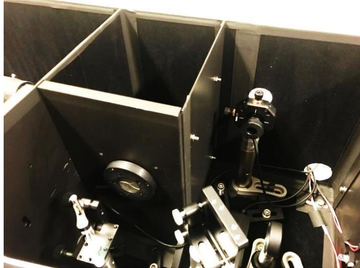
**Figure 8.11 - Shutters that equip the spectral calibration mechanical slit and the fiber bundle**
