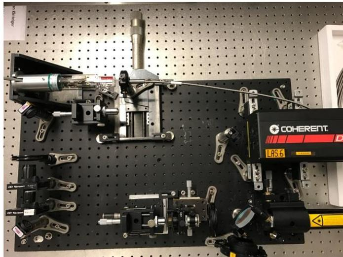
Figure 6.12 - Adapted fiber illuminating system incorporating a UNe hollow cathode lamp
