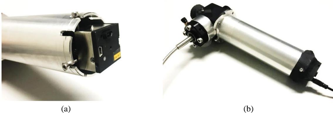
**Figure 8.21 – Camera holder (a) and adapted tracking device (b).**
