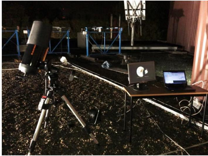
**Figure 8.22 - Observation setup installed on CSL facilities roof. A second display devoted to the tracking operation was added. The laptop was dedicated to the spectrograph control.**
