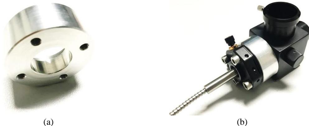
**Figure 8.16 - Connecting mechanical piece using the standard camera thread (a) and adapted fiber positioning system (b)**
