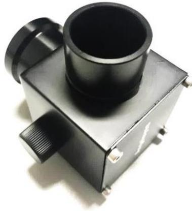
**Figure 8.15 - Flipping mirror device: the upper flange connects to the telescope, the left connecting tube intends to hold an eyepiece and the lower hidden aperture incorporates a standard thread for cameras. The small turning button activates the flipping mechanism.**
