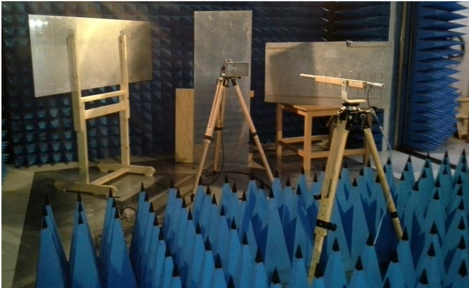
Figure 3.16: Experimental deconvolution setup for test case 4.
