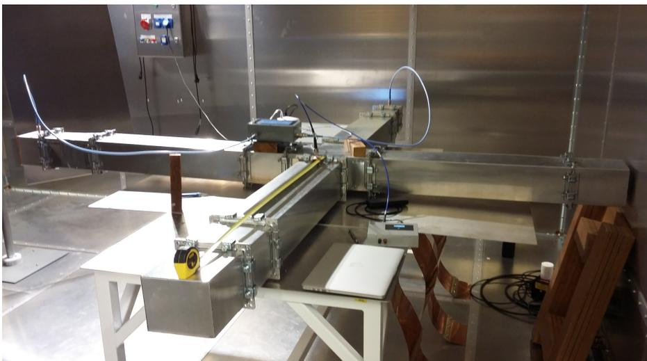
Figure B.2: Experimental setup for the waveguide network control.
