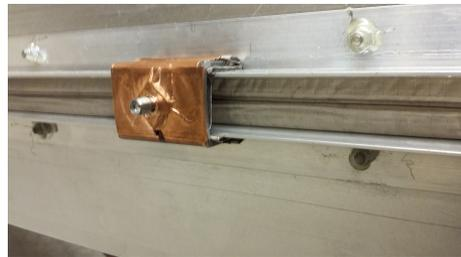
(3) RF power probe fitting the waveguide slit
