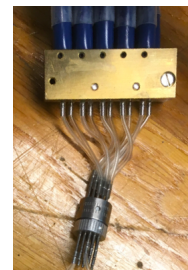
Figure 2.54 – Transducers (inside gold chamber) connected with blue VGA cables, in KTH
