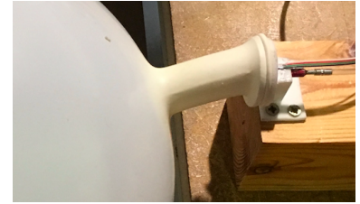
Figure A.17 – Picture of the complete setup (design 2) with 3D printed support, flush mounted transducer and PVC tube inside the ballon
