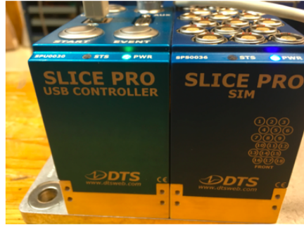
Figure 2.55 – Acquisition system Slice Pro USB controller DTS@SPU0020, Slice Pro SIM DTS@SPS0036
