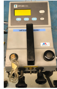
Figure 2.56 – Druck@DPI063 static calibrator in KTH, 100 [Pa] accuracy
