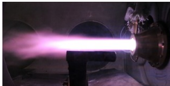
Figure 2.5: Subsonic plasma jet generated inside the Plasmatron with ICP torch of 80 [mm] diameter.
