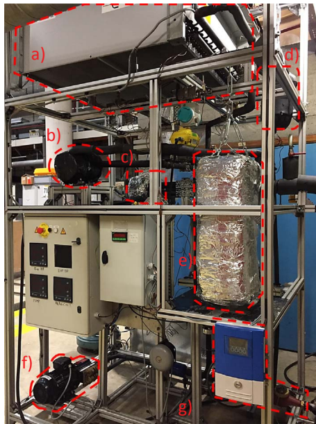
Fig. 2. Photo of the test rig. (a) Condenser (b) Expander (c) Recuperator (d) Liquid receiver (e) Evaporator (f) Pump (g) HTF flow meters.
