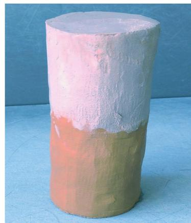
*Parallel and series specimens used for the triaxial test in this study*
