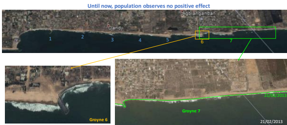
At the scale of a groyne, positive effect to the West but negative effect to the East
