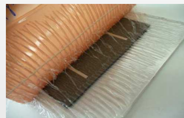
Figure 7: Overview of the removal of conductive backsheet from module, in which thermoplastic as encapsulant was applied
