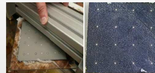
Figure 8: Separating solar cell from glass sheet for thermoplastic-based module. The separated cell is shown on the right
