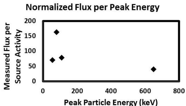
Fig. 7. Detector efficiency as a function of peak energy.
