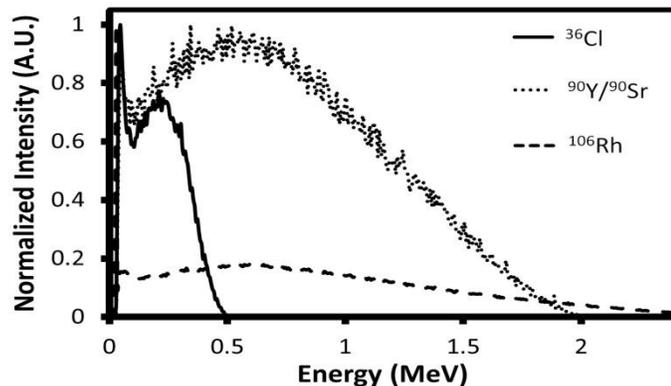
Fig. 6. Measured energy spectra of the electrons behind the cold plate used in MAJIS setup, electrons from  $^{147}\text{Pm}$  source are completely absorbed in the cold plate.
