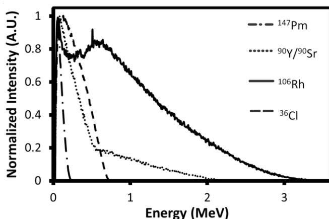
Fig. 1. Measured energy spectra of the electrons from the four radioisotopes sources.
