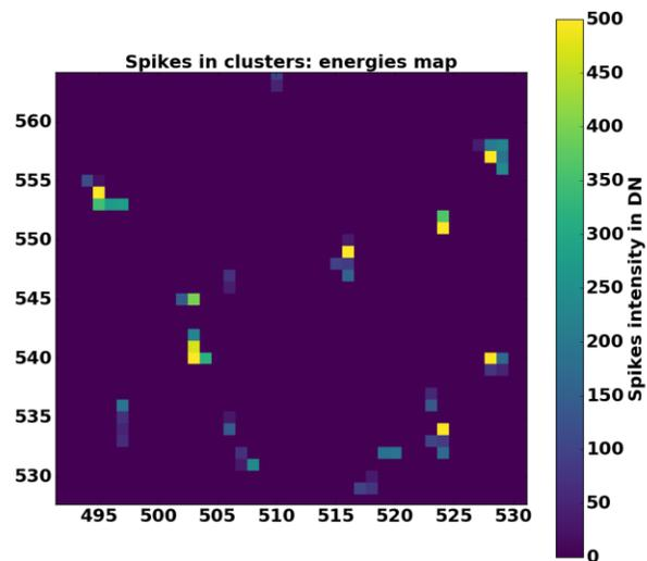
Fig. 4. Example of spikes clustering observed in a subsection of the detector for  $^{36}\text{Cl}$  source with  $T = 90\text{ K}$ , and integration time of 1s.
