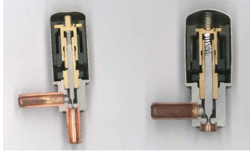
Figure 5: Cut expansion valves
