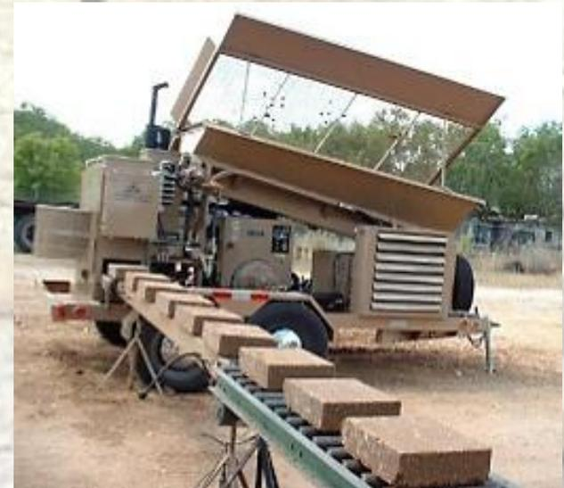
**Compressed Earth Brick (CEB):** compacted earth, achieved using manual or mechanical presses.
