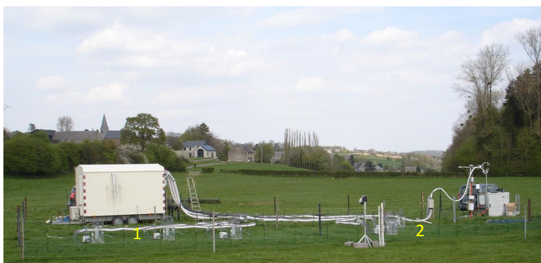
Figure 2.3: Grassland patches (1 and 2) in the DTO site separated by barbwire. Three automated soil enclosures in patch 1 and 3 in patch 2 are installed for the measurement.
