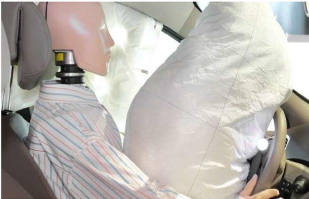
Measure shock due to accident for airbag system
