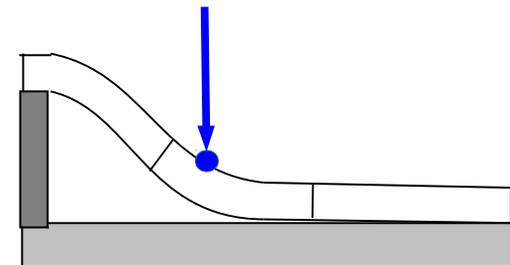
Progressively unloading and resulting stiction configuration
