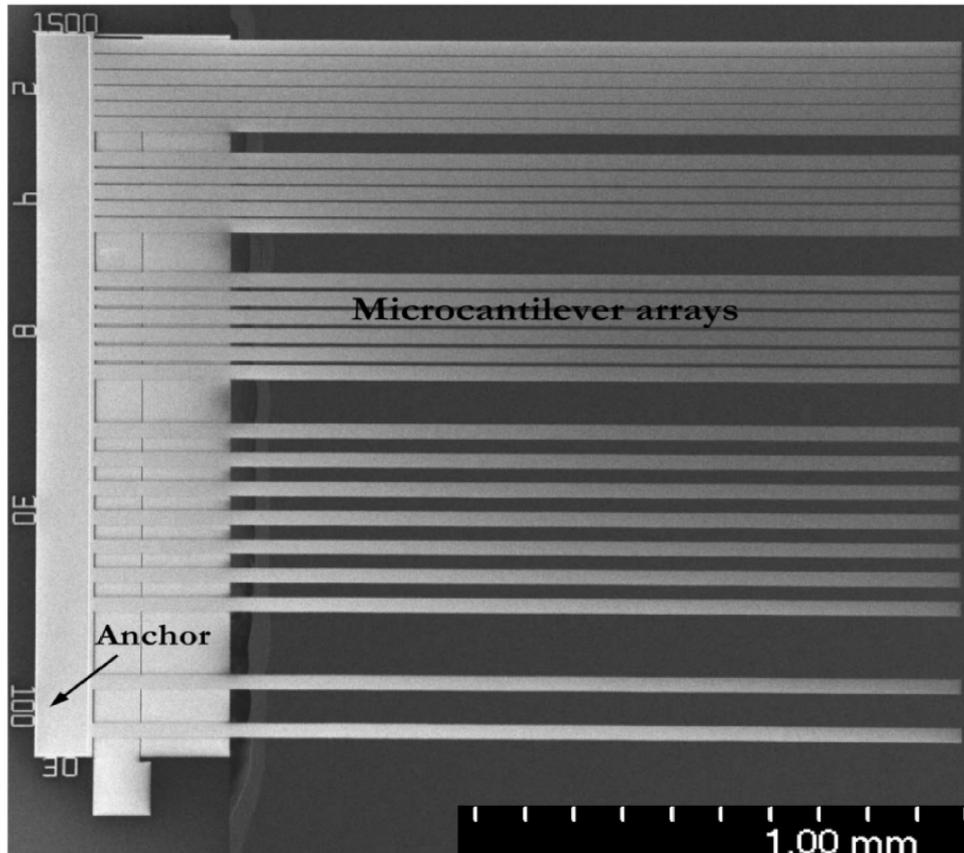
Micro-cantilever beam arrays
