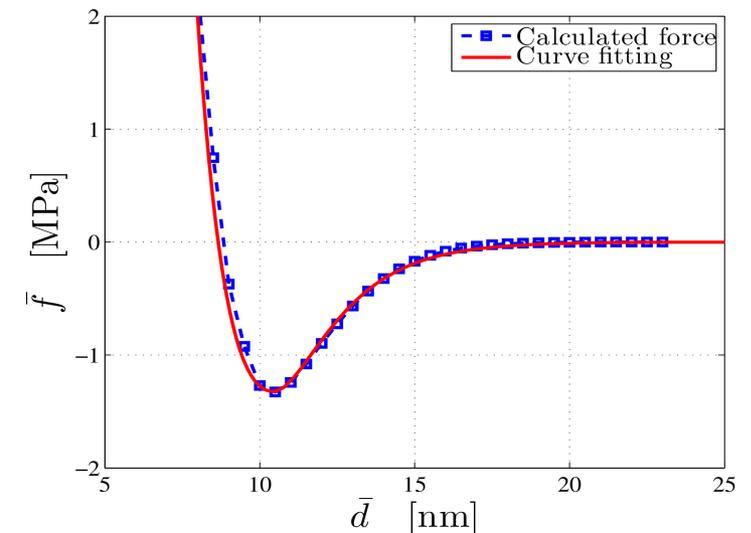
Apparent adhesive forces vs contact distances
