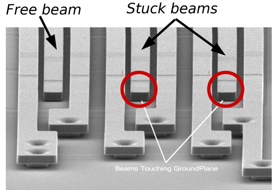
*Stiction failure in a MEMS sensor*
