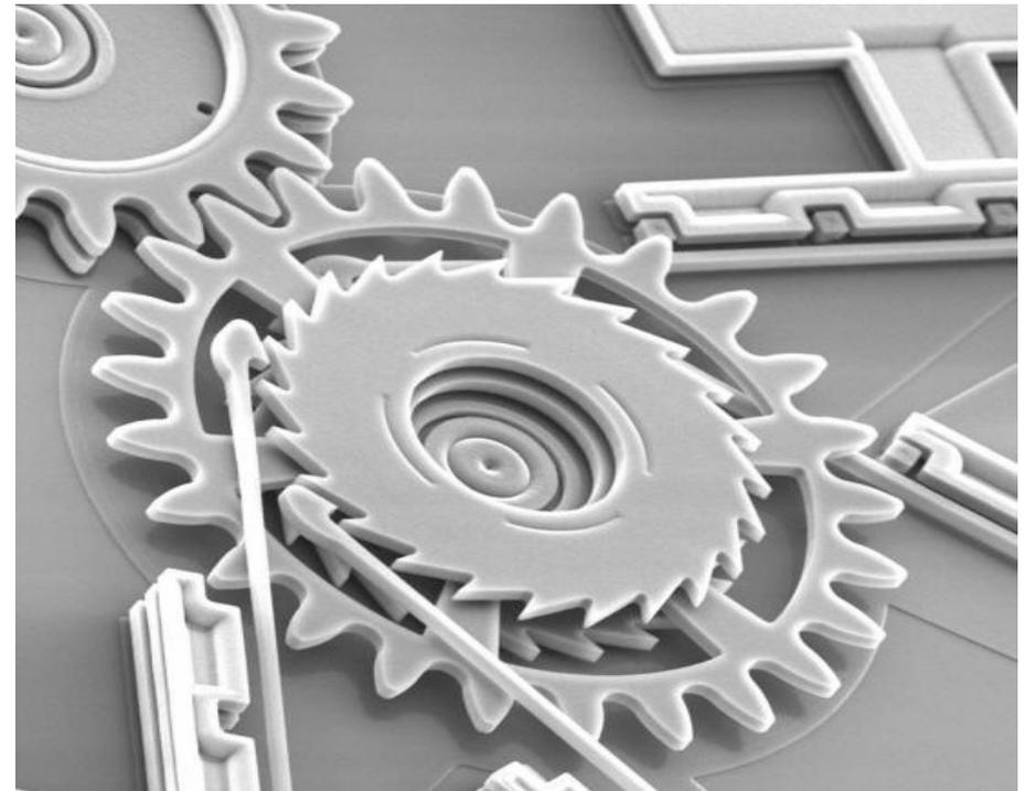
SEM image of a micro-gears system
