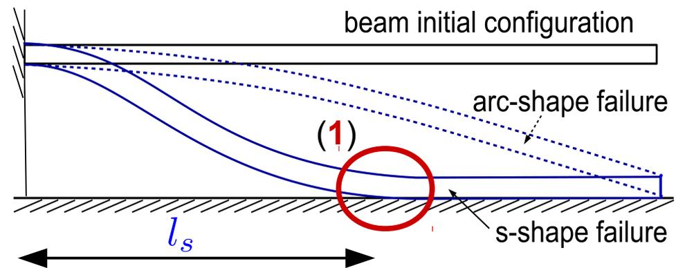
Stiction configurations of micro beam to its substrate
