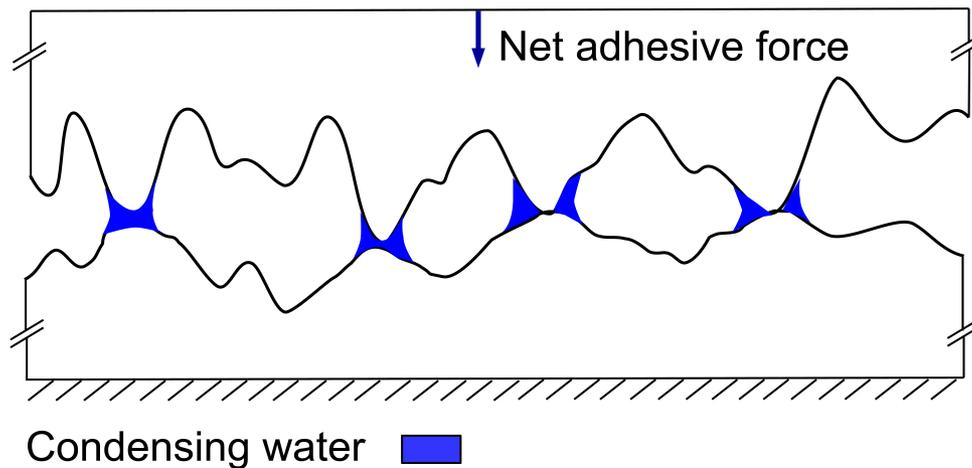
Adhesion of two contacting rough surfaces
