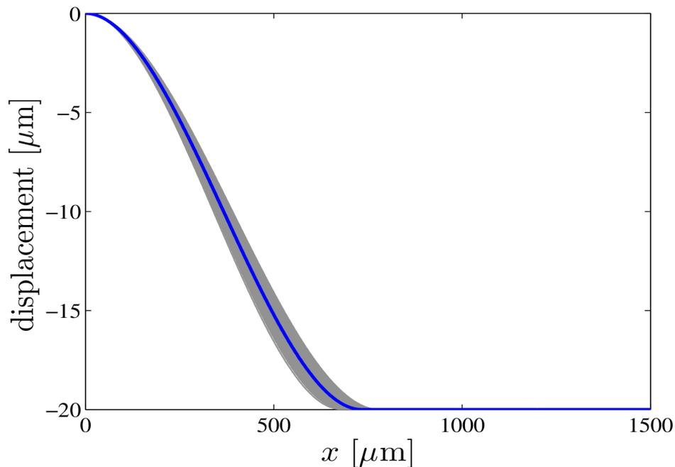
Collection of 1000 realizations of S-shape failure stiction beams (stochastic model-based method)
