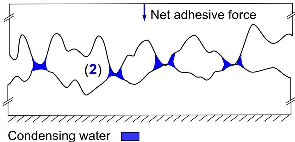
Adhesion of two contacting rough surfaces
