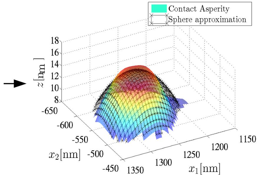
*i*-th identified contacting asperity, its spherical approximation
