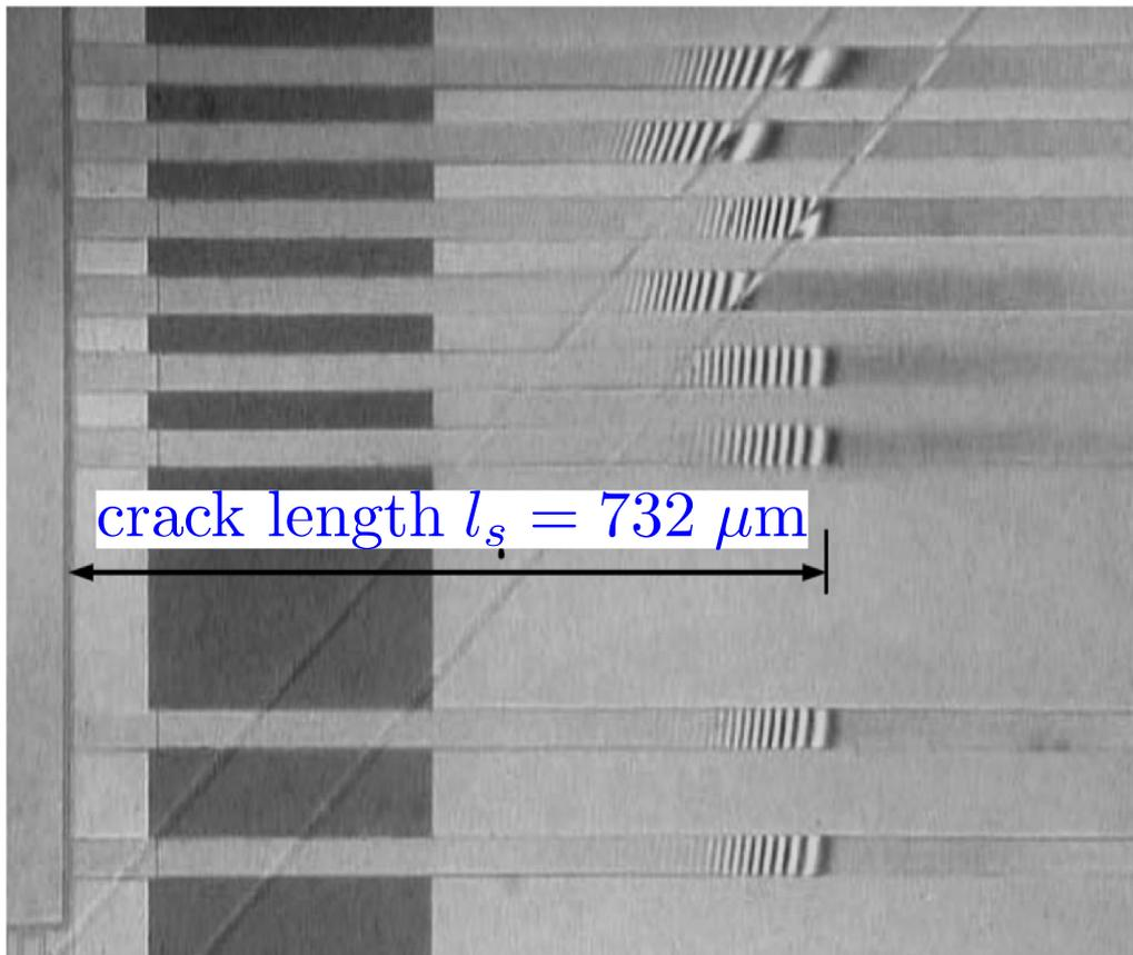
Interferometric image of beams undergoing stiction failure (top view) [Xue et al 2008]
