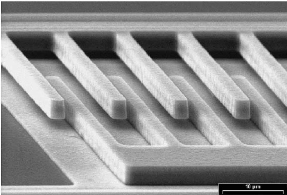
Stiction failure of comb drive
