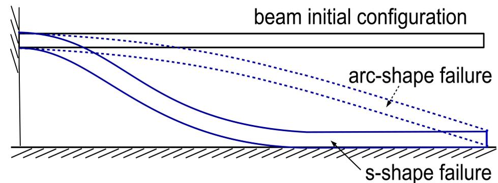
Stiction configurations of micro beams to its substrate
