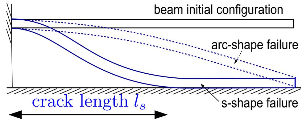
Stiction tests to measure crack length
