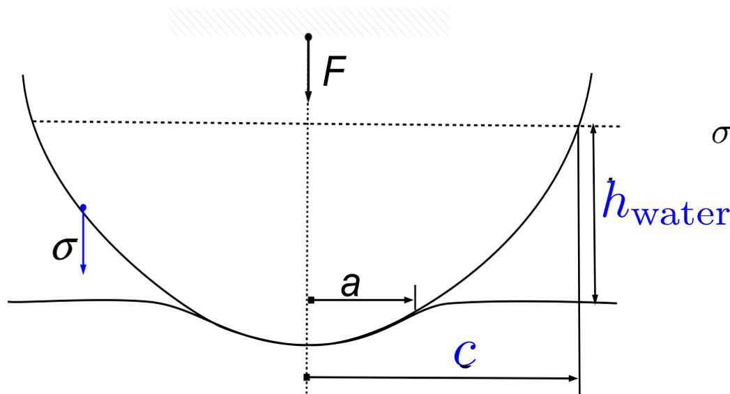
$$\sigma = \begin{cases} \Delta P & \text{if } 0 < h \leq h_{\text{water}} = 2r_K ; \\ 0 & \text{if } h > h_{\text{water}} = 2r_K \end{cases}$$
