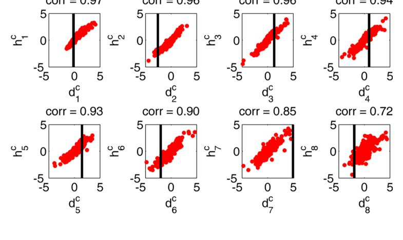
ERT data are used to forecast the spatial distribution of temperature in the aquifer. The correlation is high since data and forecast are colocated. The posterior distribution of temperature is validated direct measurements piezometers within the ERT panel.
