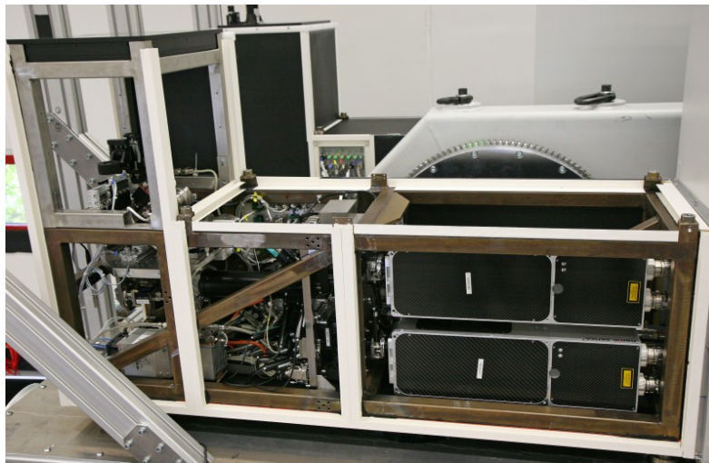
Fig. 3. Picture of one of the ARGOS laser boxes (The outer insulation panels are partially removed).
