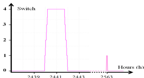
Figure 4 Different cases of switching from TRNSYS simulations. At left the window switches from clear to dark, maintains at dark state and switches from dark to clear. At right the window switches from clear to the first intermediate state and switches back to the clear state.
