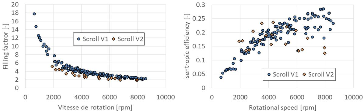
Figure 6: Performance of the scroll expander a) Filling factor and b) isentropic efficiency.
