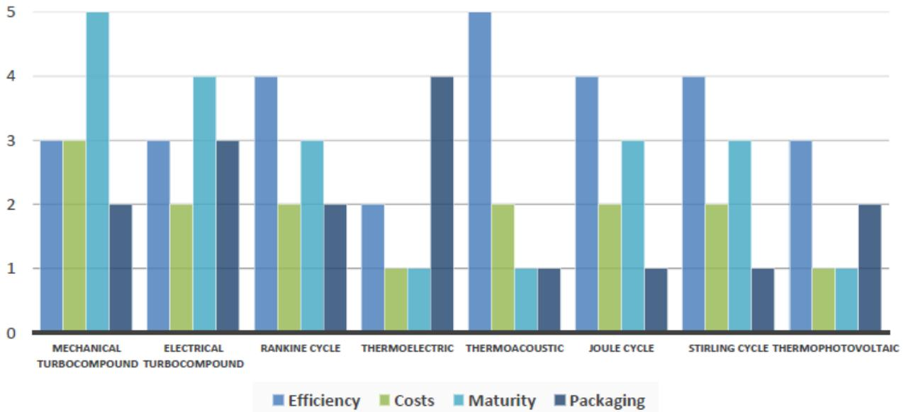
Fig. 1. Comparison of different technologies for waste heat recovery on exhaust gases [10].
