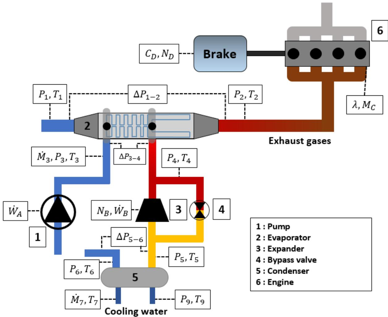
Fig. 2. Hydraulic scheme of the Rankine cycle connected to the exhaust gases of the engine
