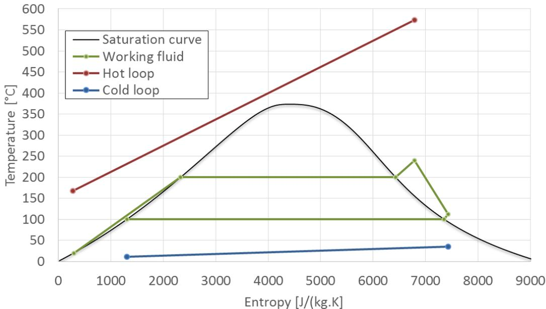
Figure 7. T-s diagram of the Rankine cycle.
