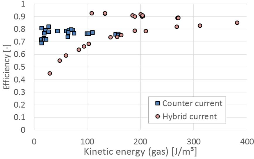
Figure 4: Evaporator efficiency
