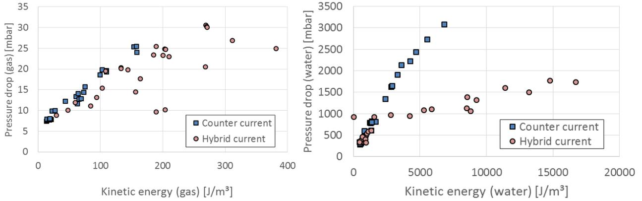
Figure 5: Pressure drop of the evaporator: a) Exhaust gas side b) Water side
