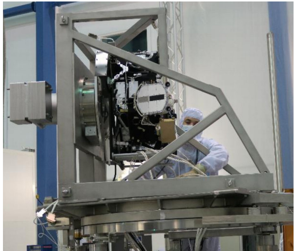
Fig. 16 ICON FUV mounted on its side on the articulating cradle inside the vacuum chamber. Turret and contamination cover door are nearest to the reader
