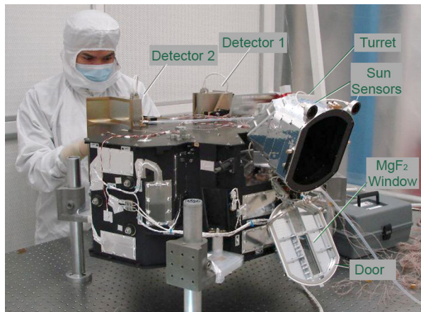
Fig. 8 A view of the ICON FUV instrument on the bench
