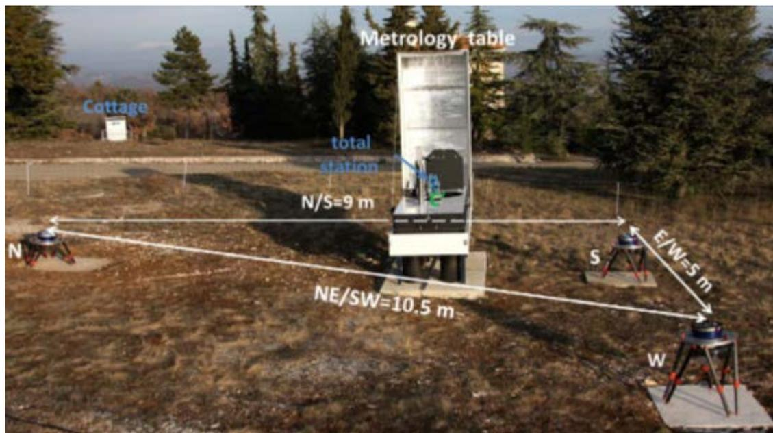
Figure 20-3: We see on this picture the three mirrors and baselines of the Carlina prototype, built at the Haute-Provence Observatory. The table of metrology has been used to align the whole system (the primary mirrors, metrology and focal gondola).
