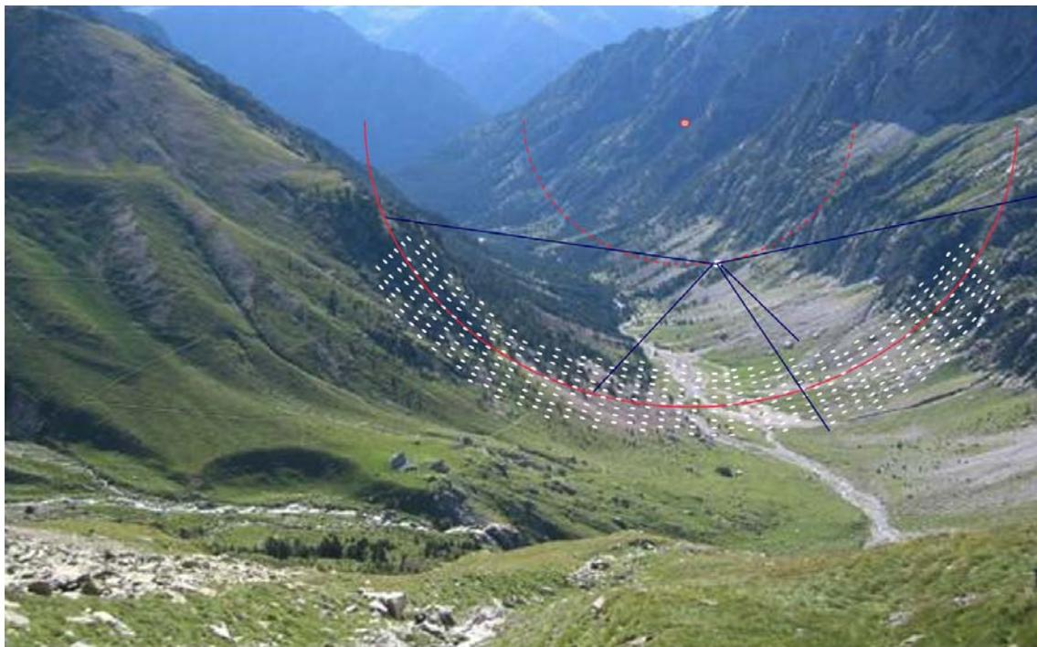
Figure 20-5: Representation of the diluted M1 mirror of the Ubaye Carlina hypertelescope prototype with the focal gondola suspended to a cable crossing the valley and connected to six cables wires to adjust translation and position to form the direct image.
