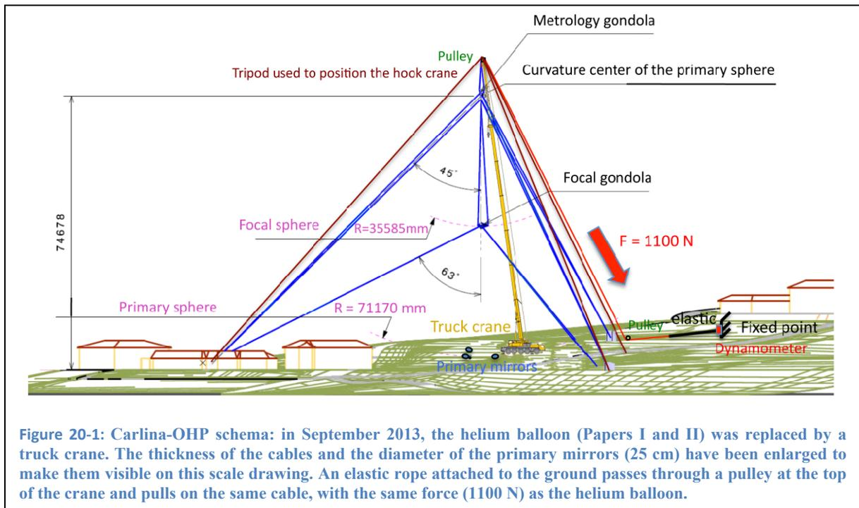
**Figure 20-1: Carlina-OHP schema: in September 2013, the helium balloon (Papers I and II) was replaced by a truck crane. The thickness of the cables and the diameter of the primary mirrors (25 cm) have been enlarged to make them visible on this scale drawing. An elastic rope attached to the ground passes through a pulley at the top of the crane and pulls on the same cable, with the same force (1100 N) as the helium balloon.**
