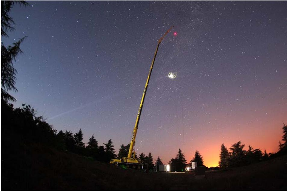
Figure 20-2: On this figure, we see the crane that is carrying a metrology gondola (red point at the summit of the crane) at the curvature center of the diluted primary mirror (71 m above the ground), and the focal gondola (enlightened in white) 35.5 m above the ground. Three primary mirrors are around the table of metrology on the ground (see also Figure 20-3).
