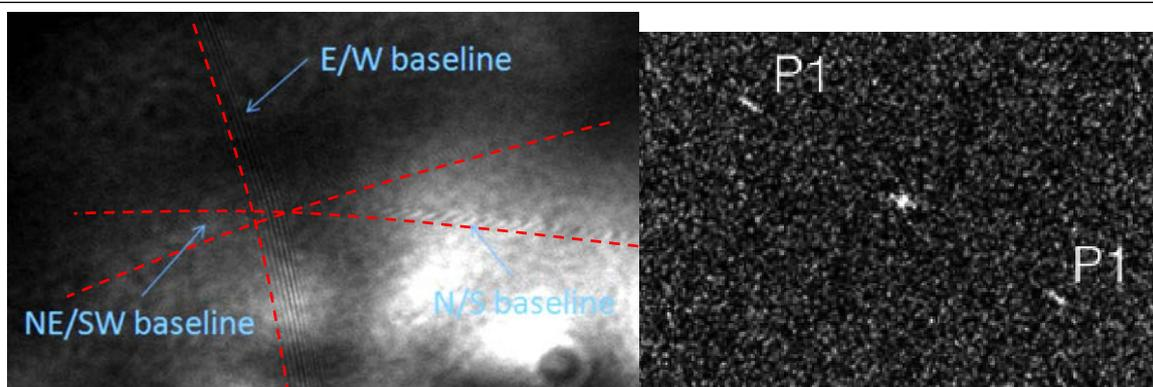
Figure 20-4: Left: Metrology fringes obtained with the Carlina OHP prototype. The red dashed lines indicate the trace of the oscillations of the fringes. Right: Square modulus of the Fourier transform of the stellar fringes recorded on Deneb with a photon-counting camera. We see the fringe peaks of the 5m baseline (P1 mark).
