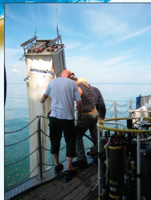
Recovery of a multi-net for plankton analysis in the Baltic Sea during a cyanobacteria bloom.
