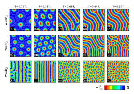
In-plane distributions of the condensate density for film thicknesses  $w=4\xi_0,\ 6\xi_0$ , and  $8\xi_0$  [ $\xi_0$  the Cooperpair radius] and temperatures  $T/T_c=0.76,0.73,0.68,0.64,0.6$ . White points (circles) in the blue background mark centers of vortices. The lattices of superconducting islands can be seen in panels (a), (b), (f), and (g). Stripes and labyrinths are in (c)-(e), (h)-(j), and (k), (l). Giant vortices and vortex clusters are in panels (m)-(o).
