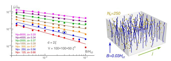
Critical current  $j_c$  as a function of field B for different defects densities  $n_p=N_p/V$ , with V the simulation volume. The power  $\alpha$  is extracted from a linear fit (lines) in the log-log representation. For the encircled point, the vortex configuration is shown.
