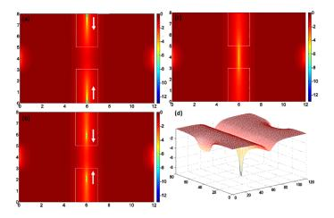
Map of the  $\log(\psi)$  during the annihilation process of a KVA pair. From (a) to (c) is shown the motion sequence of the pair. In (d) is shown a surface  $\log(\psi)$ . Note that  $\psi$  remains very small along the line of the KVA motion in a instant just before the annihilation.
