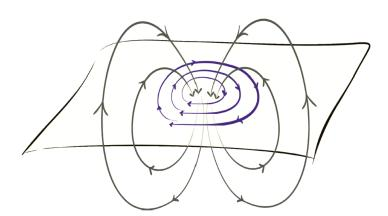
The topologically stable states are formed by closed magnetic field streamlines that pierce the layer twice and give rise to circulating surface currents.
