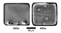
Nanocrystalline vortex matter nucleated in field-cooling processes in Bi<sub>2</sub>Sr<sub>2</sub>CaCu<sub>2</sub>O<sub>8- $\delta$ </sub> cuboids with 30  $\mu$ m sides and 2  $\mu$ m thickness. Magnetic decorations were performed at 4.2 K and at applied fields of 20 (left panel) and 40 Oe (right panel).
