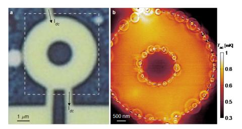
(a) Optical image of hBN/graphene/hBN structure patterned into a washer shape (bright). (b) Thermal image of the outlined area in (a) in presence of  $I_{dc}$ = 6  $\mu$ A at 4.2 K. The necklace of rings reveals the presence of resonant states along the edges of graphene that serve as local centers of energy dissipation.
