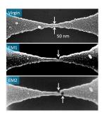
Ex-situ scanning electron images illustrating the shrinking of the constriction due to subsequent electromigrations. The upper panel corresponds to the virgin sample with arrows indicating the approximate width. The middle and lower panels represent, respectively, the sample after the first and the second run of electromigration with arrows pointing out the created voids in the junction.
