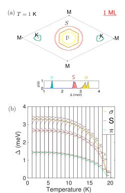
(a) Superconducting gap spectrum of one monolayer MgB $_2$  at 1 K, calculated using anisotropic Eliashberg theory, and plotted on its Fermi surface. The distribution of the gaps  $\rho(\Delta)$  shows three separate gaps on the  $\pi$ , S and  $\sigma$  sheets. (b) The evolution of the gap spectrum with temperature. The gap averages per sheet are also plotted, showing the persistence of three-gap superconductivity over the entire temperature range.
