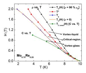
H-T phase-diagram of Mo<sub>0.75</sub>Re<sub>0.25</sub> alloy superconductor
