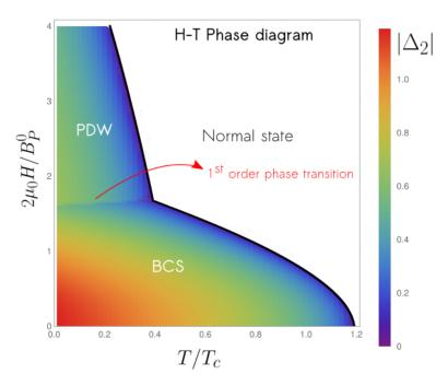
Typical magnetic field—temperature phase diagram of a parity-mixed three-layer system obtained within a Ginzburg-Landau theory.  $\Delta_2$  shows refers to the order parameter of the middle layer. A first order phase transition separates the low field BCS from the high field PDW region. Here  $T_c$  is the superconducting critical temperature of a single layer, which shows that a three-layer system has its critical temperature increased.
