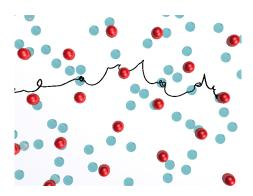
Real-space image of skyrmions (dark red dots) driven through randomly arranged pinning sites (light blue dots) in a plastic flow phase. The trajectory of a single skyrmion is highlighted, and reveals spiraling motions of the skyrmions inside the pinning sites.
