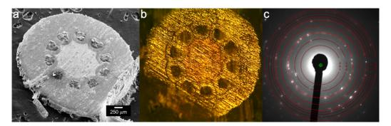
(a). SEM image of a slice of superconductor cable of ten  $MgB_2$  filaments. (b). Optical image showing a detail of superconducting nuclei and individual filaments. (c). Diffraction pattern of  $MgB_2$  precursor powder. Related planes have been indexed in some rings at the pattern.
