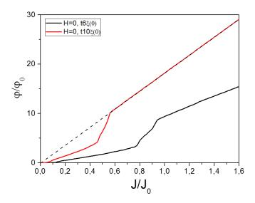
Voltage as a function of the applied current density without external magnetic field. (a) Constriction due to two blind slit (b) Constriction crossing all sample width.
