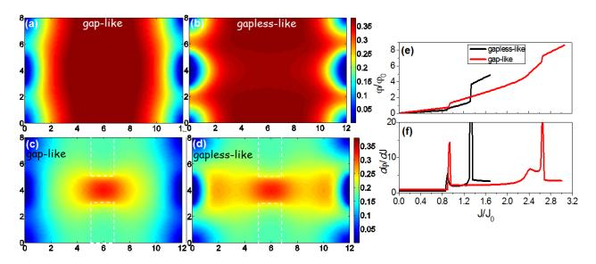
Map of the modulus of the superconducting current,  $J_s$ . (a) and (b) homogeneous gap-like and gapless-like samples, respectively. (c) and (d) gap-like and gapless-like samples with constriction, respectively. (e) is the  $\varphi(J)$  for the gap and gapless-like samples and (f) is the differential resistance.
