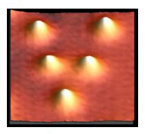
A vortex pattern 'V' short for vortex is assembled by using the STM tip.
