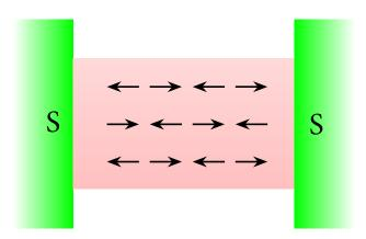
The Josephson junction S-AF-S with metallic antiferromagnet between two BCS superconductors.
