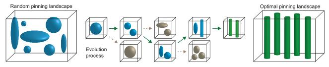
Sketch of the evolution process. A randomly generated pinscape is 'mutated' by adding/removing, moving, and reshaping defects. After each mutation the configuration with maximal critical current is chosen.
