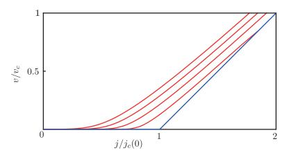
Current-voltage characteristic in the strong pinning scenario for fixed defect density  $n_p a_0 \xi^2 = 10^{-3}$  and different temperatures (from right to left)  $T/e_p = (0, \ 0.5, \ 1, \ 1.5, \ 2) \times 10^{-2}$ . The velocity axis is rescaled by  $v_c$  denoting vortex velocity at driving current  $j_c(0)$  in absence of pinning.
