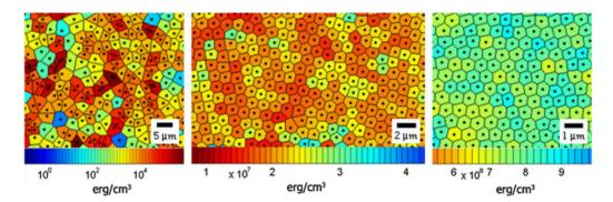
Maps of interaction vortex energies for vortex positions at the FLL (black dots at images). Results come from Bitter decoration experiments performed on YBCO single crystals at 16.5 Oe, 33 Oe and 66 Oe (respectively) under field cooling conditions. Changes in the FLL order are clearly exposed.
