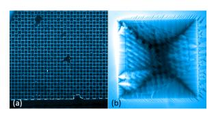
(a) MO image of Nb-NdFeB at 10 K, 59 Oe, showing TMP chessboard pattern in NdFeB. (b) MO Image of Nb-Py at 6 K, 59 Oe, showing smooth flux penetration in Nb guided by chessboard pattern imprinted in Py.
