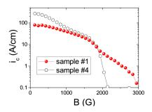
Persistent current measured in a Niobium slab for after two different surface treatments. Note the collapse of the surface critical current for  $B > Bc2 \approx 0.19T$  for the sample labelled  $\sharp 4$  (smooth surface).
