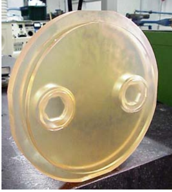
Fig. 5: M1 flight and spare models before extraction from their master (courtesy AMOS SA)
