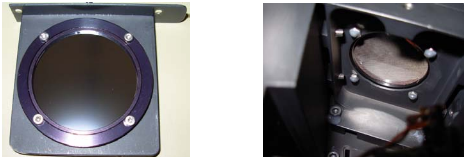
Fig. 8. SWAP front and rear aluminum foil filters
