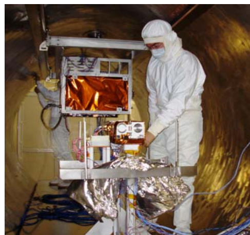
Fig. 16. SWAP environmental qualification (vibrations and thermal vacuum) in CSL facilities (Liège, B)
