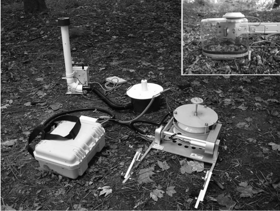
Figure 2.3 Open dynamic chamber systems from different manufacturers. PP-Systems CFX-1 at the back and ADC SRS-1000 in the small figure. Automatic closed dynamic system Li-Cor Li-8100 chamber at the front is based on closed dynamic technique.
