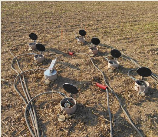
Figure 1. Gas measurement device: one set consisting of 8 chambers.
