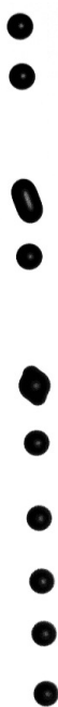
Figure 7. Example of merged drops in the case of a forced break up regime at 160 mm from the injector tip.
