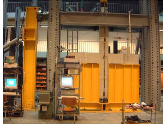
Figure 3-5. Test configuration adopted at the University of Liege (masonry “infills” are in yellow).
