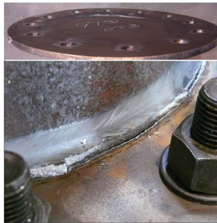
Crack in flange of specimen L1
