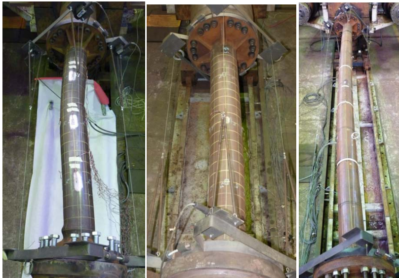
Figure 133 Columns after axial compression tests: column Cs1, Cs1-b and C11 (left to right)
