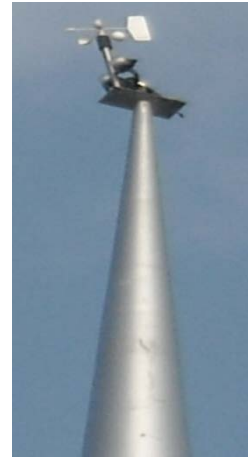
Figure 93 Anemometers: (a) 2 m below the foot deck (b) At the mast (height about 40 m)
