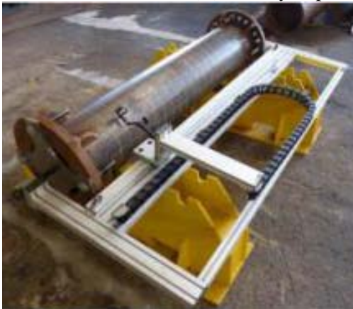
Figure 129 Frame arranged on short specimen measuring phase on cross section of a short specimen
