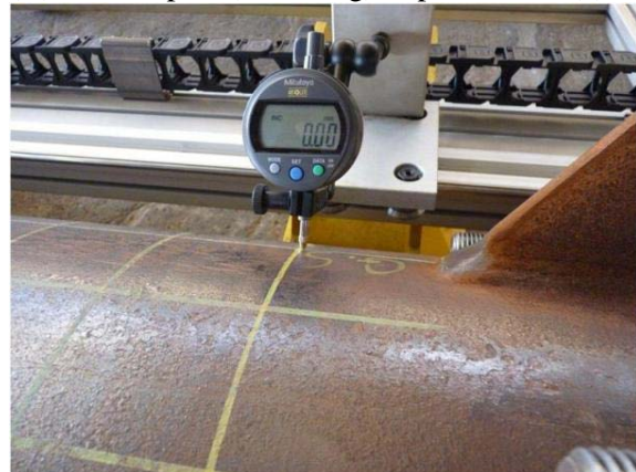
Figure 129 Frame arranged on short specimen measuring phase on cross section of a short specimen
