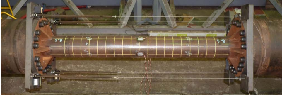
Figure 128 Full-scale column testing arrangement
