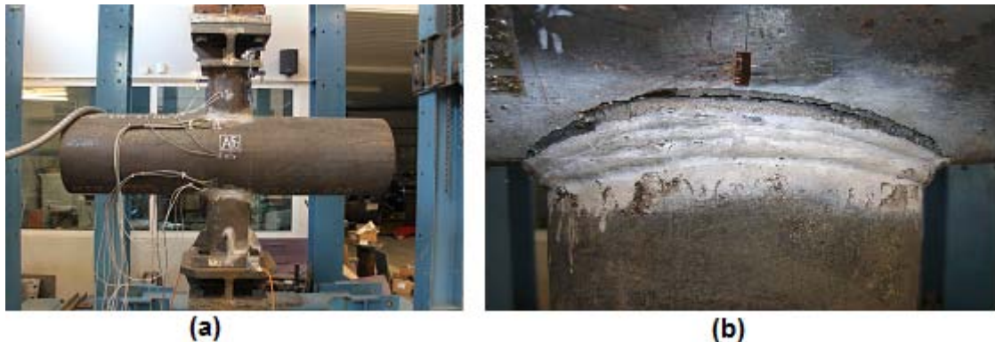
Figure 47 Tested specimen under axial cyclic loading; (a) general set-up , (b) fatigue crack at weld toe (chord saddle location)
