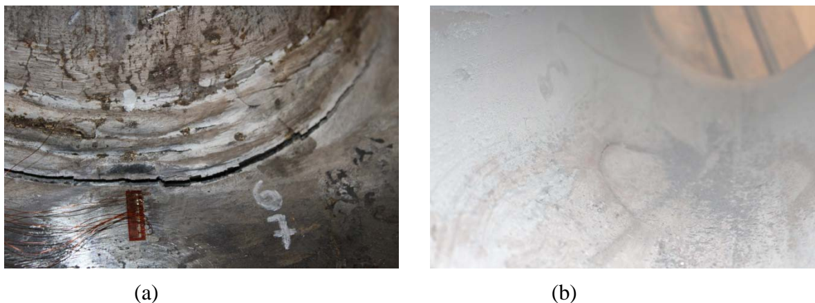
Figure 147 Fatigue crack of axial loading specimen; (a) external view of crack at chord saddle, (b) internal view of through-thickness crack development.
