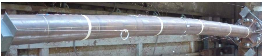
Figure 134 Columns after combined load test: a) specimen Cs3-13; b) specimen C13-75
